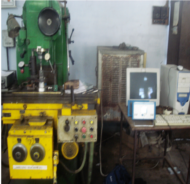
Figure 4.12 Complete setup for friction welding
