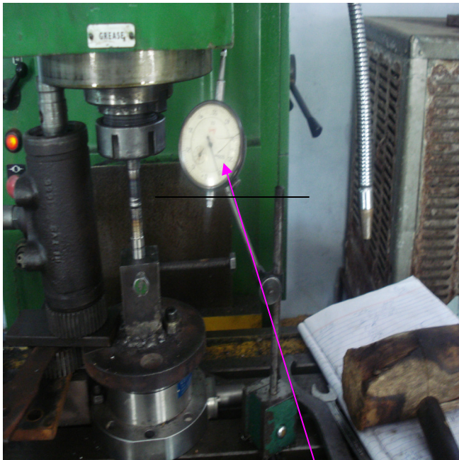
Figure 4.5 Dial indicator used to control the burn off length
