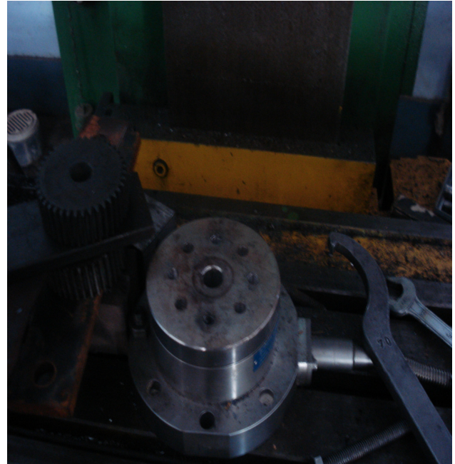
Figure 4.4 Piezoelectric Load Cell used to plot graphs
