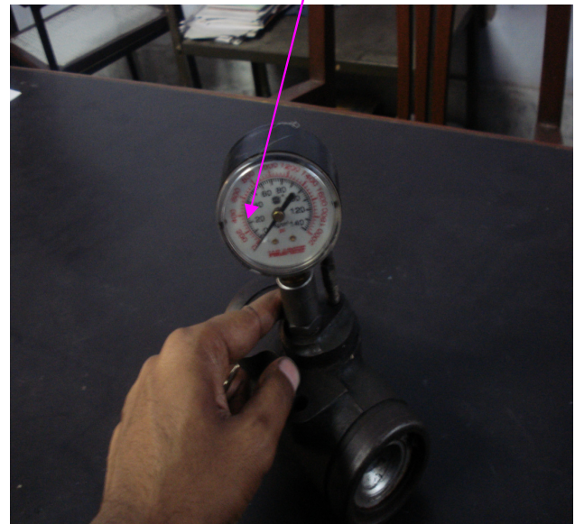
Figure 4.2 Pressure gauge used during friction welding to control the force
