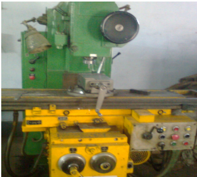
Figure 4.1 Vertical Milling Machine used for friction welding
