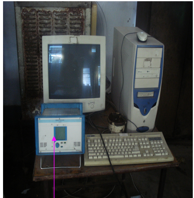
Figure 4.6 Computer and Display of Piezoelectric Dynamometer
