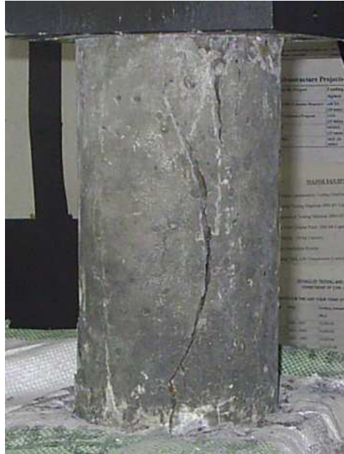
Picture 1: Failure of cylinder having no fly ash at room temperature (28 days)
