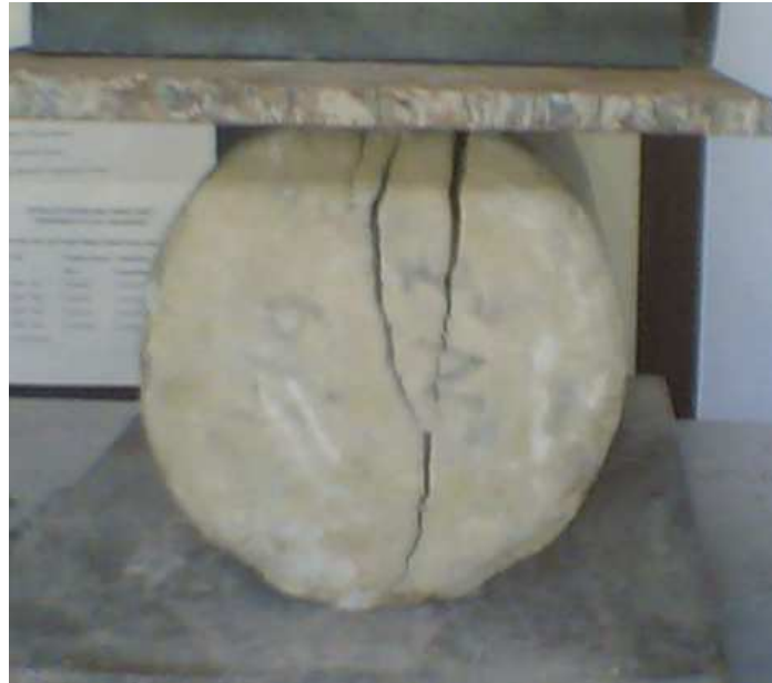
Picture 9: Splitting Tensile Failure of cylinder having 40% fly ash at room temperature (56 days)
