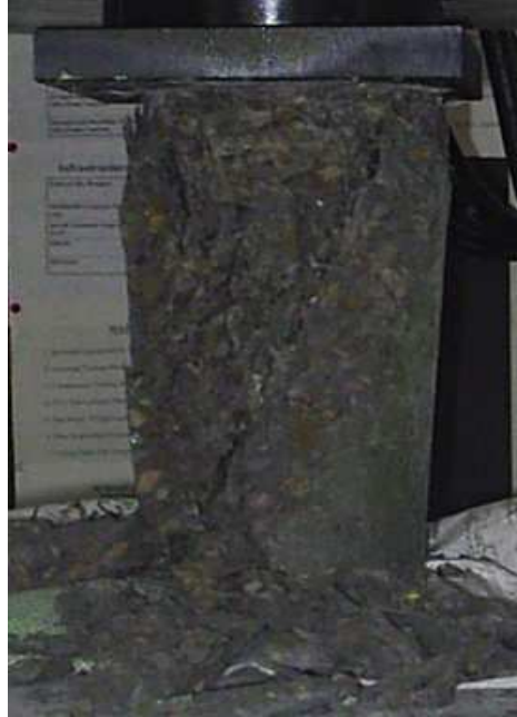
Picture 7: Failure of cylinder having 40% fly ash at 100°C (56 days)
