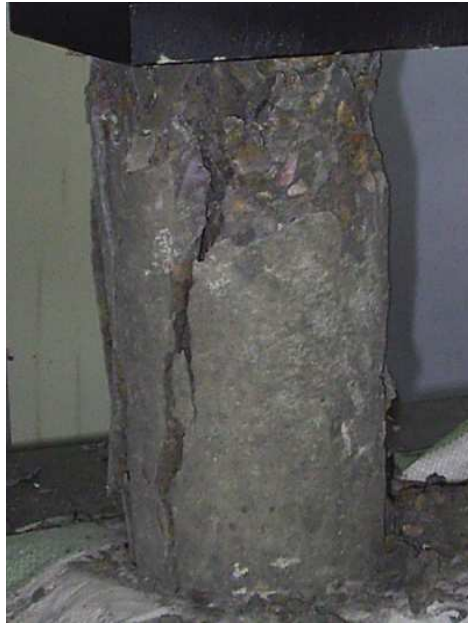
Picture 5: Failure of cylinder having 40% fly ash at room temperature (56 days)
