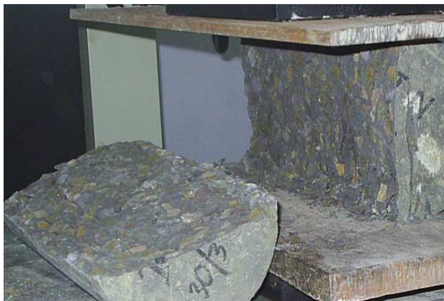
Picture 11: Splitting Tensile Failure of cylinder having 40% fly ash at 100°C (56 days)
