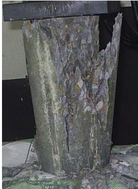
Picture 2: Failure of cylinder having no fly ash at 80°C (28 days)
