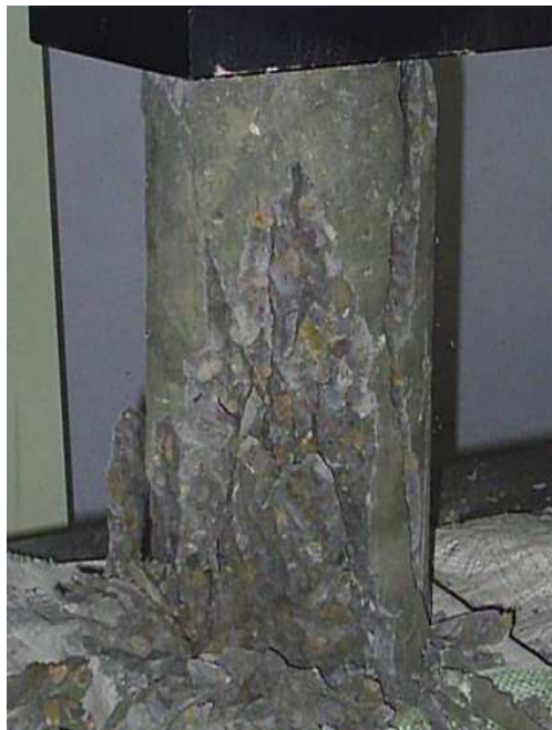
Picture 4: Failure of cylinder having no fly ash at 120°C (28 days)
