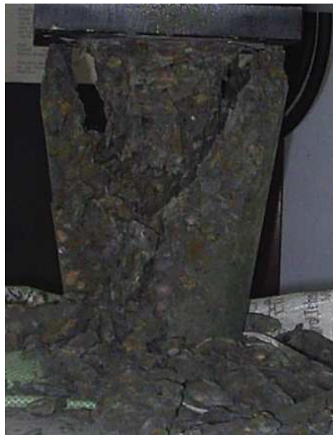
Picture 7: Failure of cylinder having 40% fly ash at 100°C (56 days)
