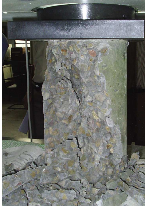
Picture 3: Failure of cylinder having no fly ash at 100°C (28 days)
