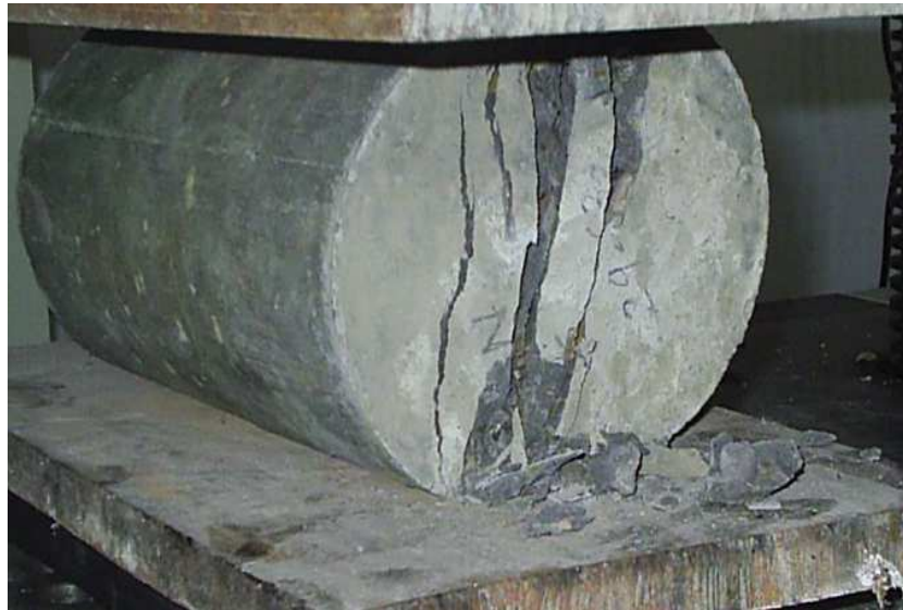
Picture 11: Splitting Tensile Failure of cylinder having 40% fly ash at 100°C (56 days)
