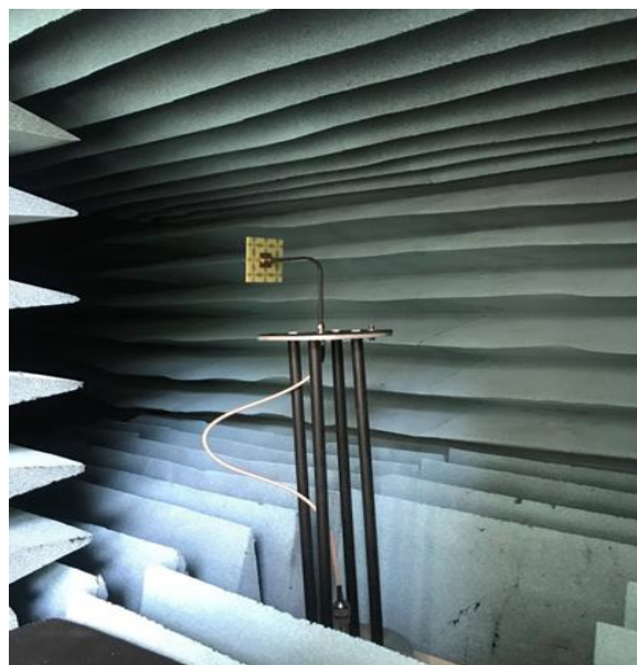
Figure5.5 Experimental Setup of coaxial fed fabricated metamaterial loaded antenna
