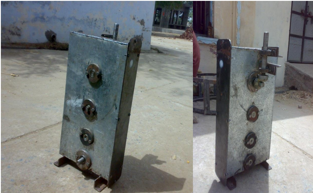
Figure: 5.3 Gear box of standalone cattle driven generator
