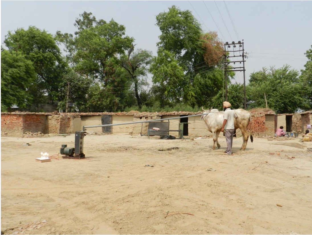
Figure: 5.5 Bullock in action; generating electricity
