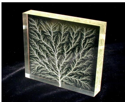
Figure 1: Fractal phenomenon, (a) frost patterns (b) pulling apart 2 glue coloured acrylic sheet (c) High voltage breakdown within a 4" block of acrylic creates a fractal Lichtenberg figure.
