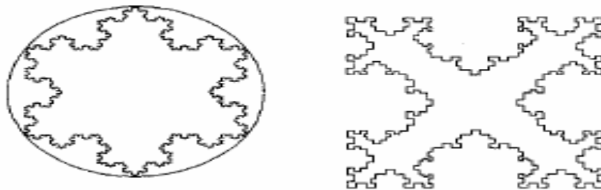
Figure 8 : Some Common Fractal Geometries Found in Antenna Application: Koch snowflakes/islands. These are used in miniaturized loop
