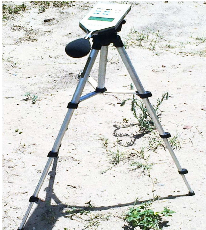
FIG.16 Sound level meter on a tripod with windscreen
