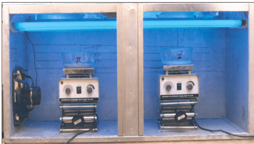
Figure 3.2: Experimental Setup consisting of UV chamber, magnetic stirrer and slurry pond reactor
