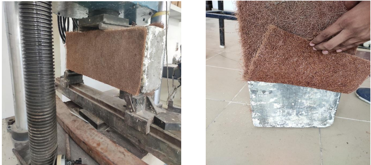
Figure 4.3: Testing of CF beam and debonding around the shear crack failure
