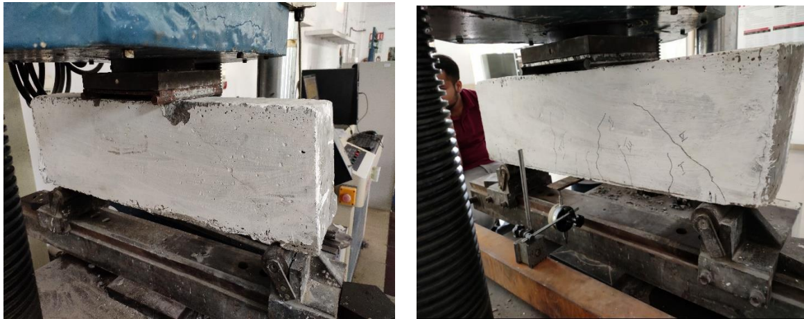
Figure 4.1: Testing of Control beam and crack pattern of control beam
