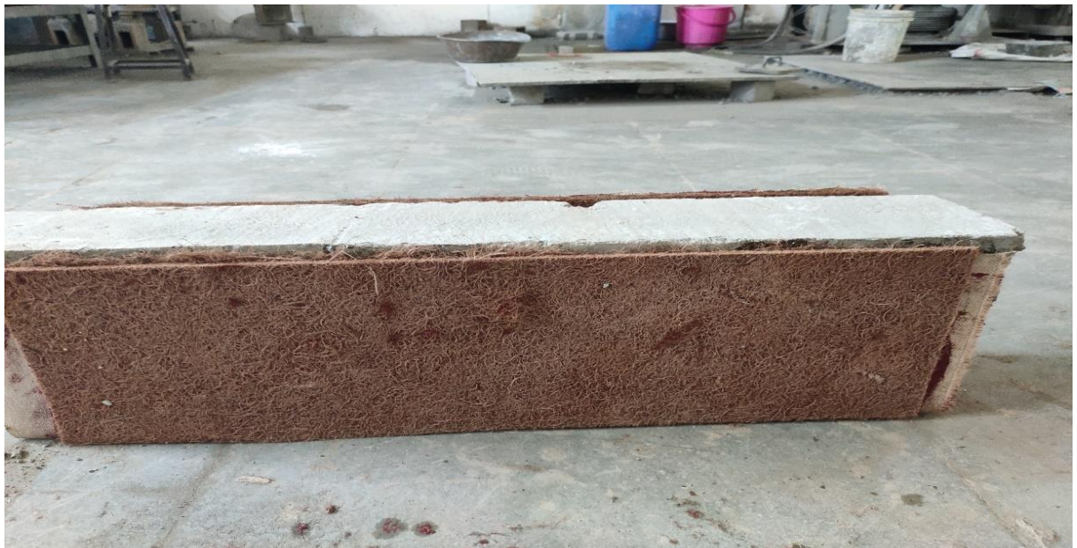
Figure 3.6 – Beam after Side face retrofitting using coir fiber
