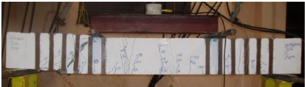
Figure 2.5: Mode of failure of Untreated jute rope fiber beam [Alam, M.A. et al. (2017)]
