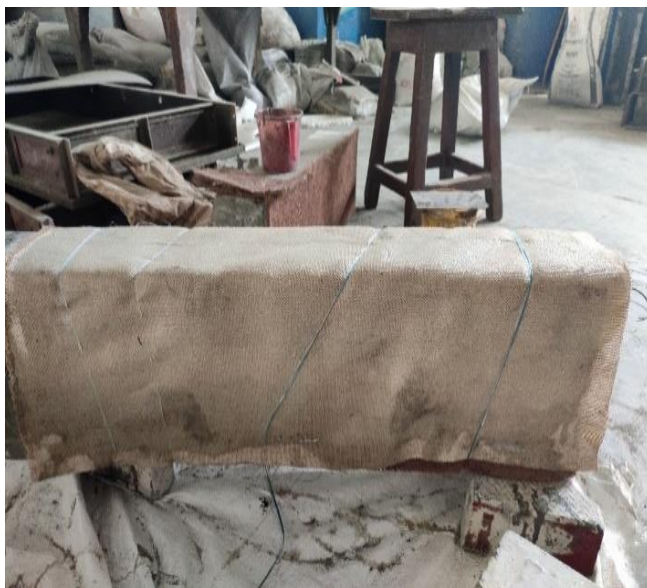
Figure 4.8: Retrofitting of CFU beam and CFU beam after shear failure
