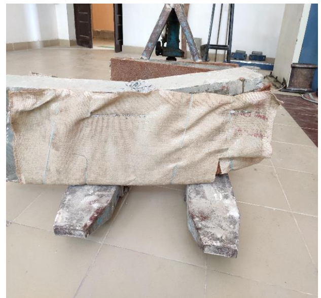
Figure 4.8: Retrofitting of CFU beam and CFU beam after shear failure
