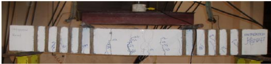
Figure 2.3: Mode of failure of Untreated jute fiber beam [Alam, M.A. et al. (2017)]
