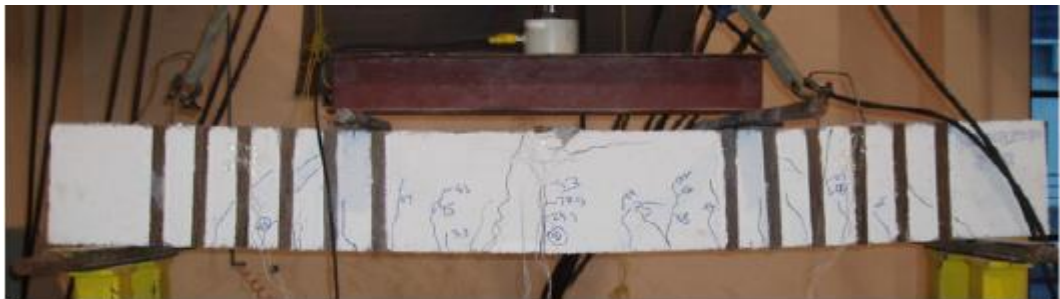
Figure 2.4: Mode of failure Untreated kenaf fiber beam [Alam, M.A. et al. (2017)]
