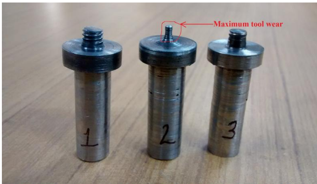
Figure 4.3: Condition of tool (after wear) (1 for Al 359 alloys, 2 for Al 359 – SiC composites, 3 for Al 359 – SiC – Gr composites)
