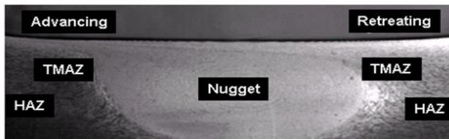
Figure 1.3 (a) Schematic diagram of micro structural zones in friction stir welds in Al (b) Micrograph showing various micro-structural zones (Threadgill, 2007)
