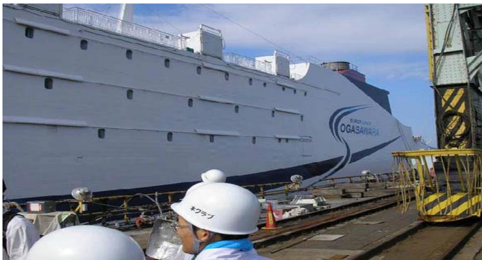
Figure 1.6 Aluminum ships constructed in Japan using FSW (Rowe and Thomas, 2006)
