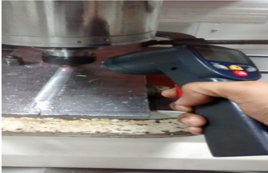
Figure 4.10: Measuring of temperature with the help of laser thermocouple
