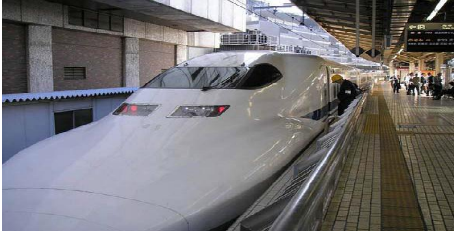
Figure 1.8 Japanese railway rolling stock fabricated from aluminum by FSW (Rowe and Thomas, 2006)
