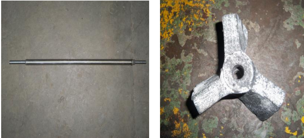
Figure 3.6: Preparation of rod and impeller for stirrer
