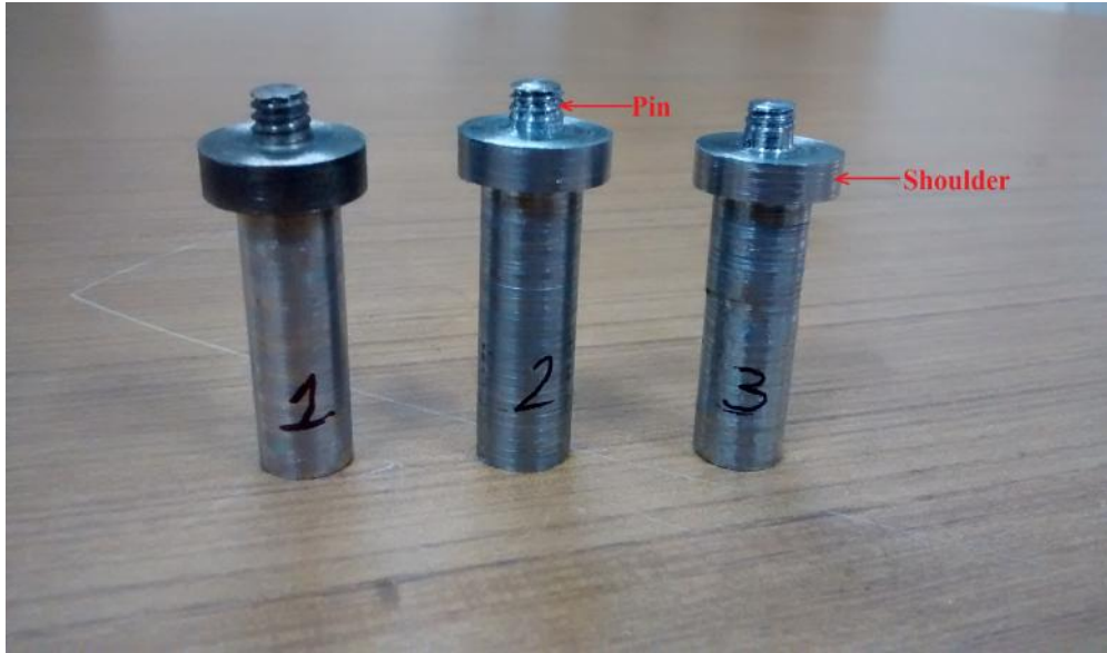
Figure 3.17: FSW tools (1 for Al 359 alloys, 2 for Al 359 – SiC composites, 3 for Al 359 – SiC – Gr composites)
