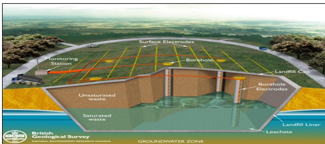
Fig 1.5: Design of Municipal solid waste landfill
