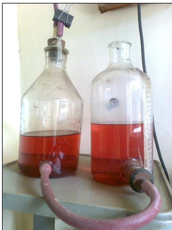
Fig 3.3: Liquid displacement method for biogas (ml) measurement.
