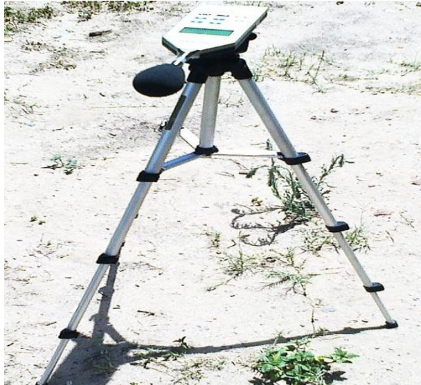
Figure 4.4 Sound level meter on a tripod with windscreen
