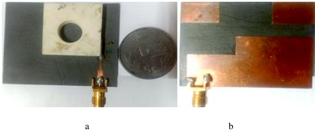
Figure 3.12: Fabricated proposed CAGRDRRA; a). Top view, b). Bottom view
