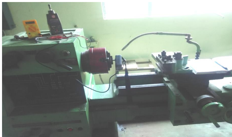
Fig. 4.6: HCG connected to Lathe machine to measure generator output
