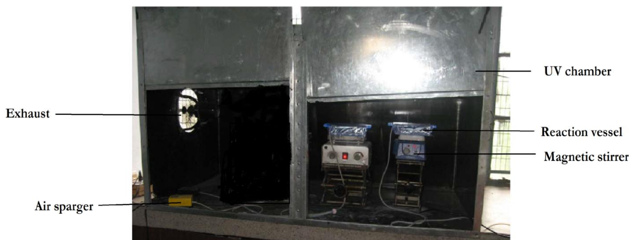
Fig 3.1 Photo reactor at lab level during photocatalytic treatment
