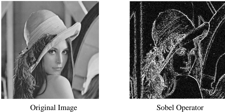
Figure 3.6 Effect of Sobel Operator on an image
