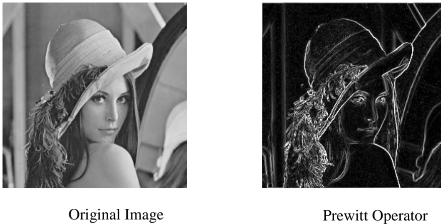
Figure 3.5 Edge enhancement using Prewitt Operator
