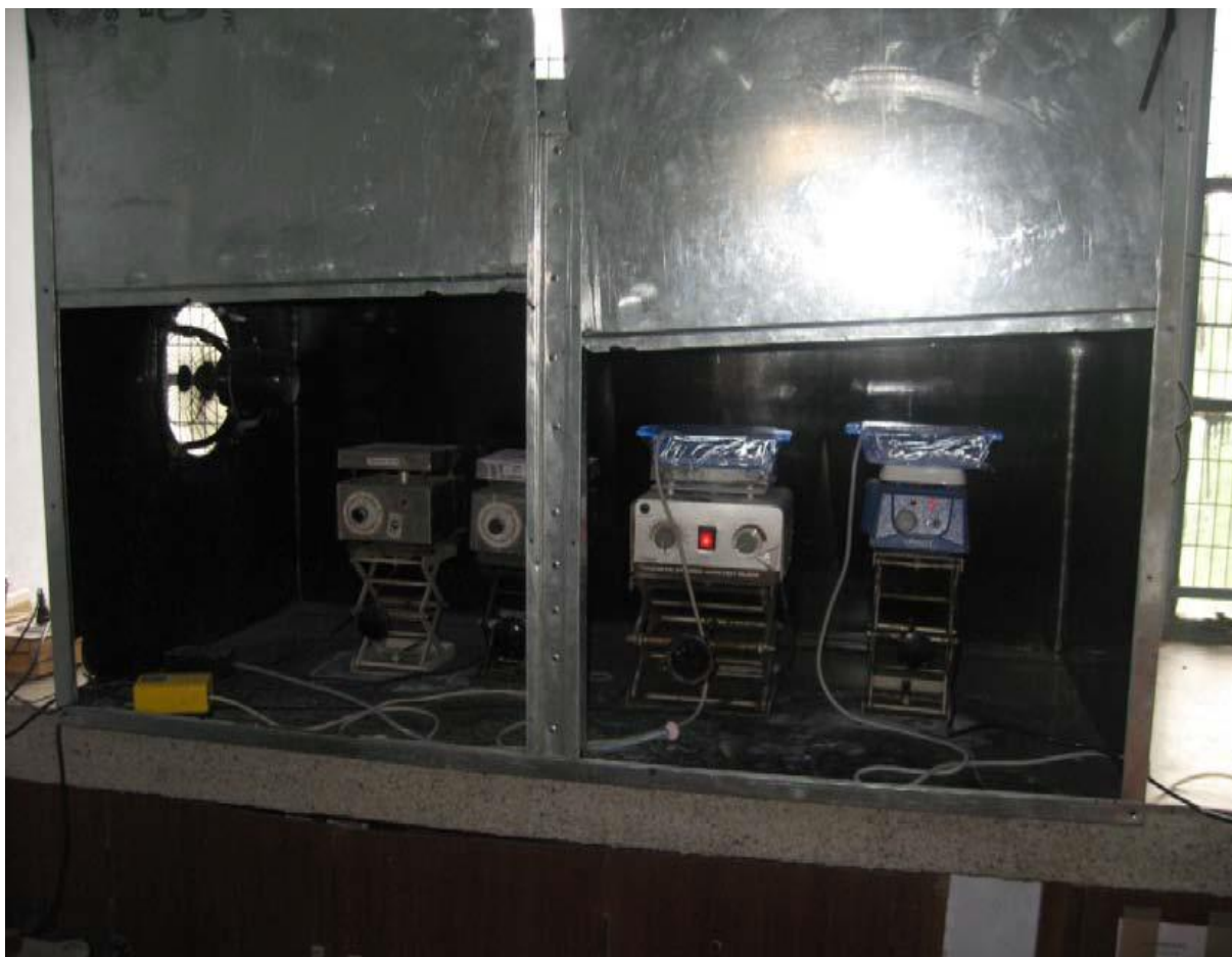
Fig 3.1 Photo reactor at lab level during photocatalytic treatment
