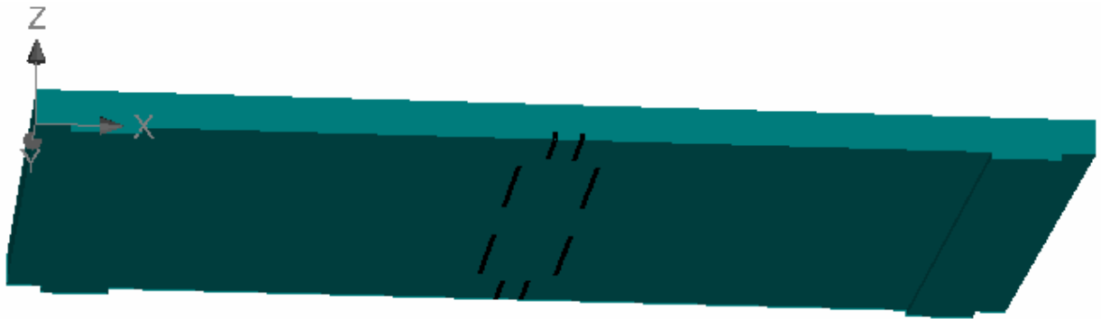
Figure 4.20 Cracks of 0.31mm width at deflection of 1.61mm
