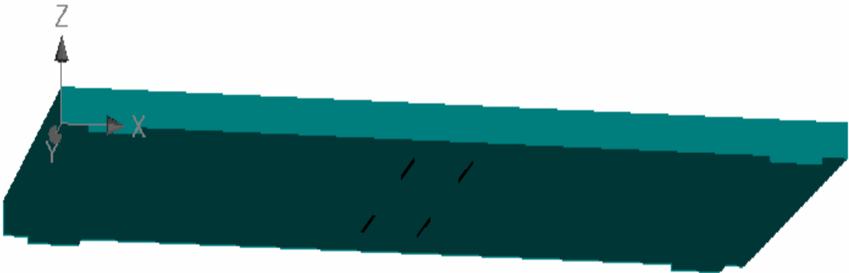
Figure 4.19 Cracks of 0.15mm width at deflection of 1.27mm
