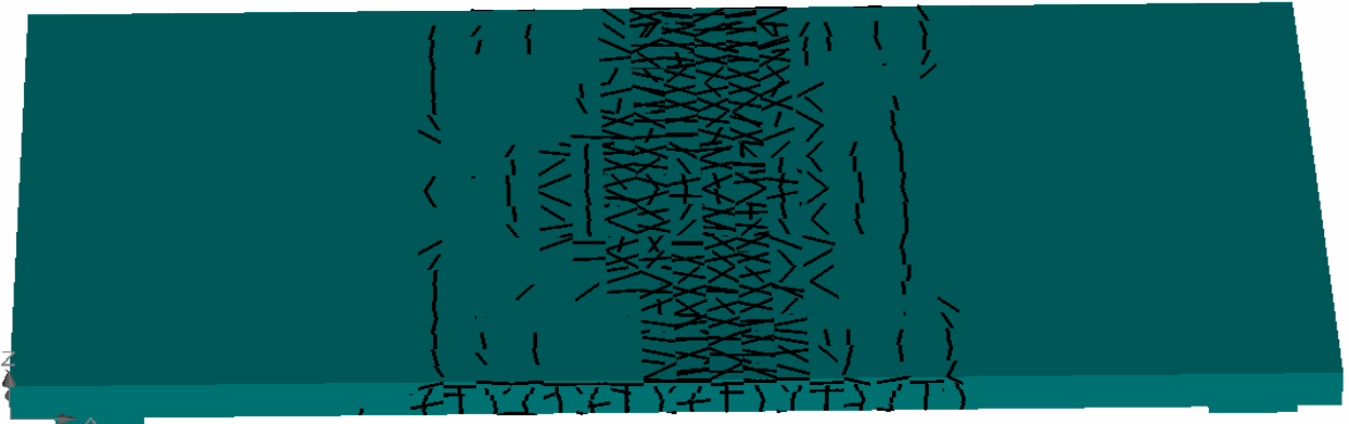
Figure 4.7 All cracks at top surface of the slab at deflection of 12.2mm
