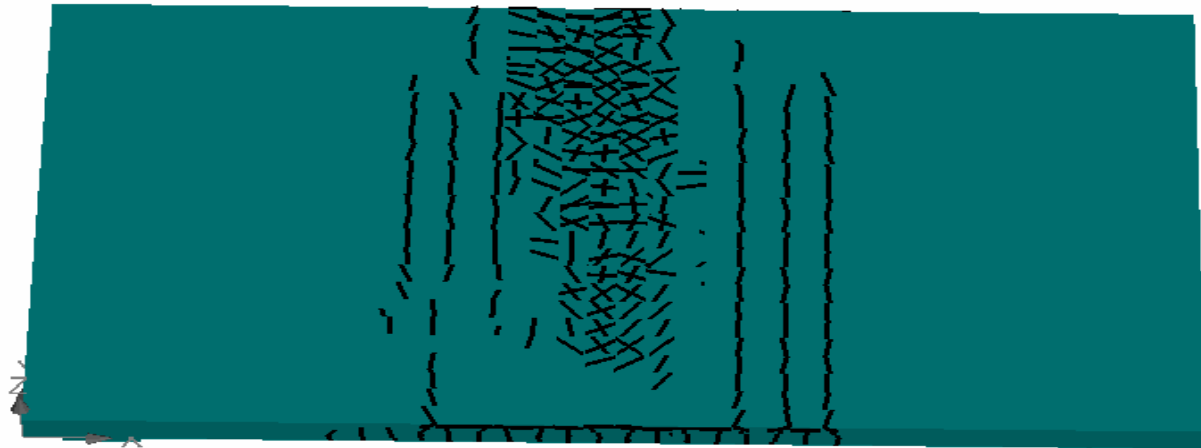
Figure 4.33 All cracks at top surface of the slab at deflection of 13.2mm
