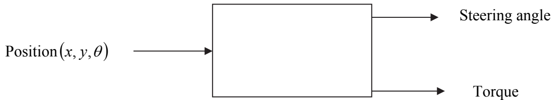
Fig. 1.2 Inverse vehicle model
