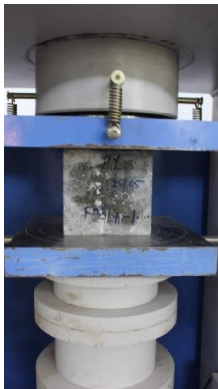
Fig 3.2: Compressive strength test setup
