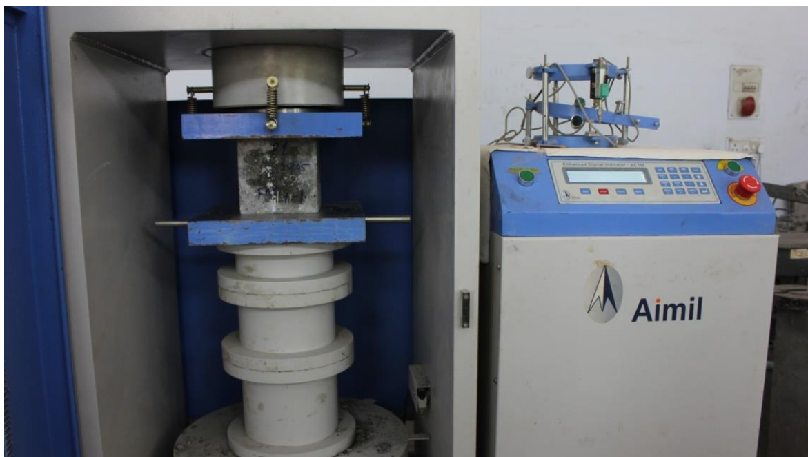
Fig 4.1: Cube under compression in Automatic Compression Testing Machine (ACTM)
