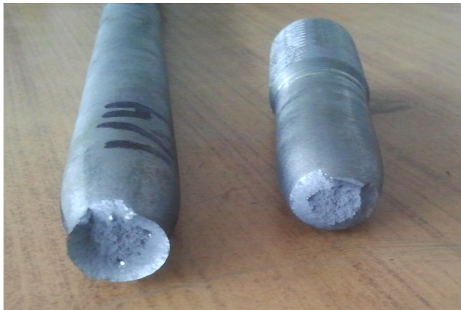
Fig. 4.20 Failed Specimen S11 after tensile test
