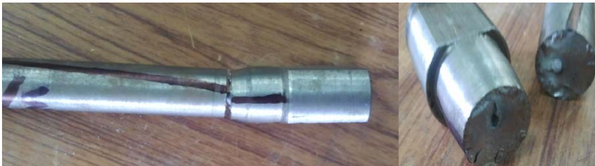
Fig. 4.7 Specimen S2 twisted to destruction to find the maximum angle of twist
