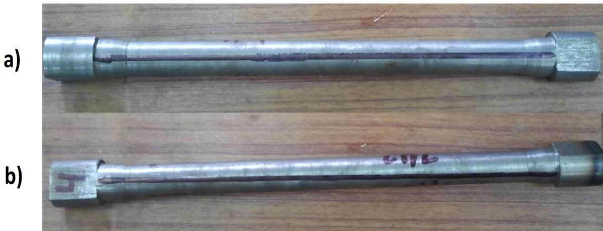
Fig.4.9 a) Healthy specimen b) Twisted Specimen 20% of max. angle of twist(50 degree)
