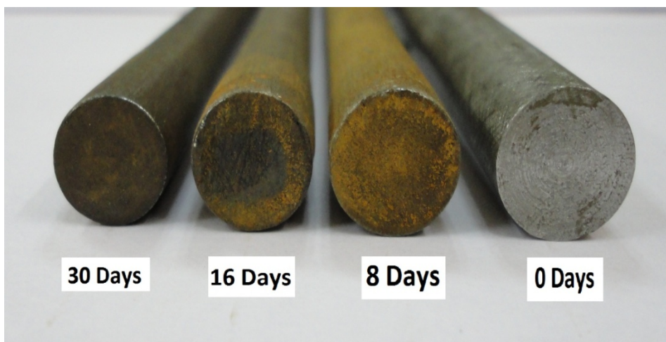
Fig. 5.14 Corroded Rods having different number of days of corrosion
