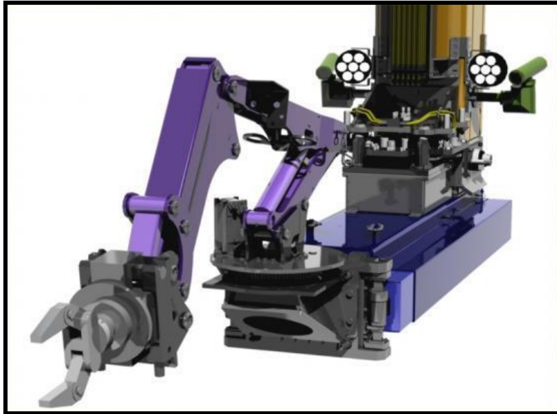
Fig. 1.3: Redundant Manipulators used in Nuclear Plants [24].
