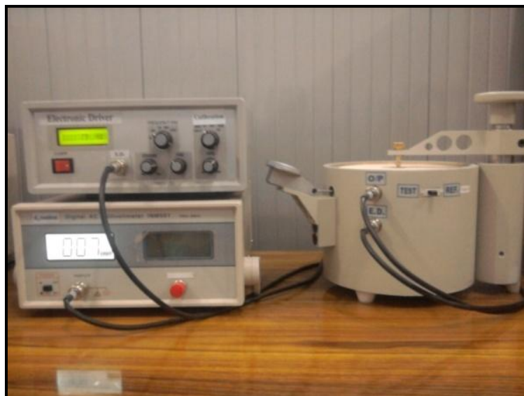
Figure 2.13 Piezo d_{33} meter
