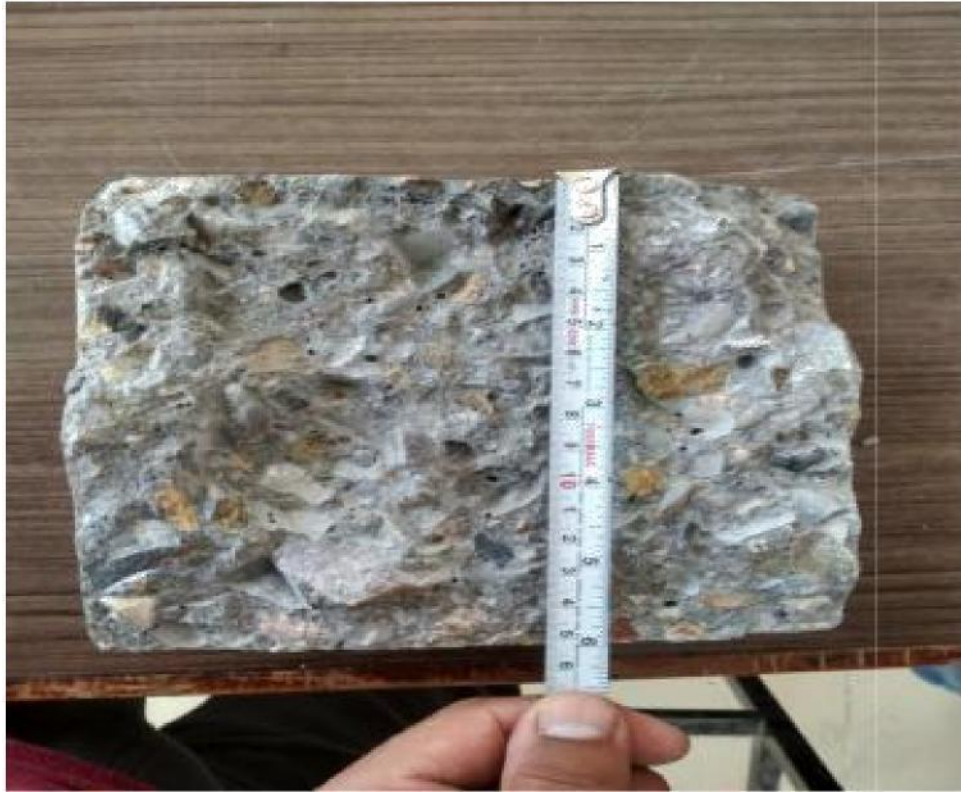
Plate 3.5: Depth of penetration of splitted concrete specimen
