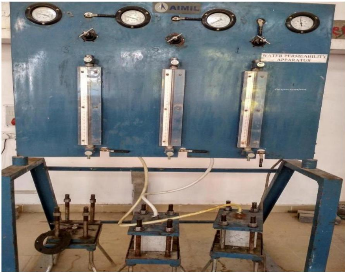
Plate 4.1: Penetration test apparatus
