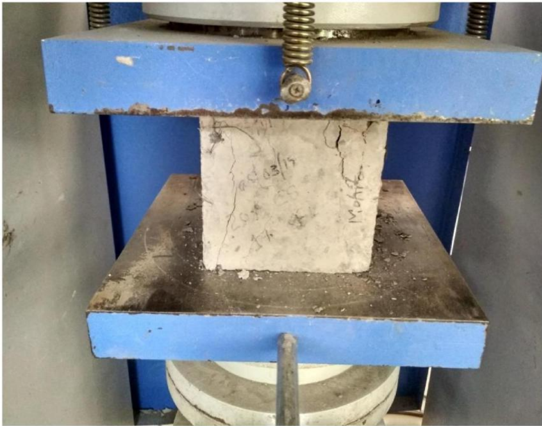
Plate 3.3: Cube compression test in Compression testing machine
