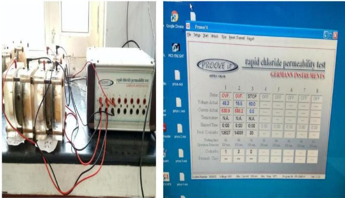
Plate 4.2: Rapid chloride permeability test apparatus and observation screen.
