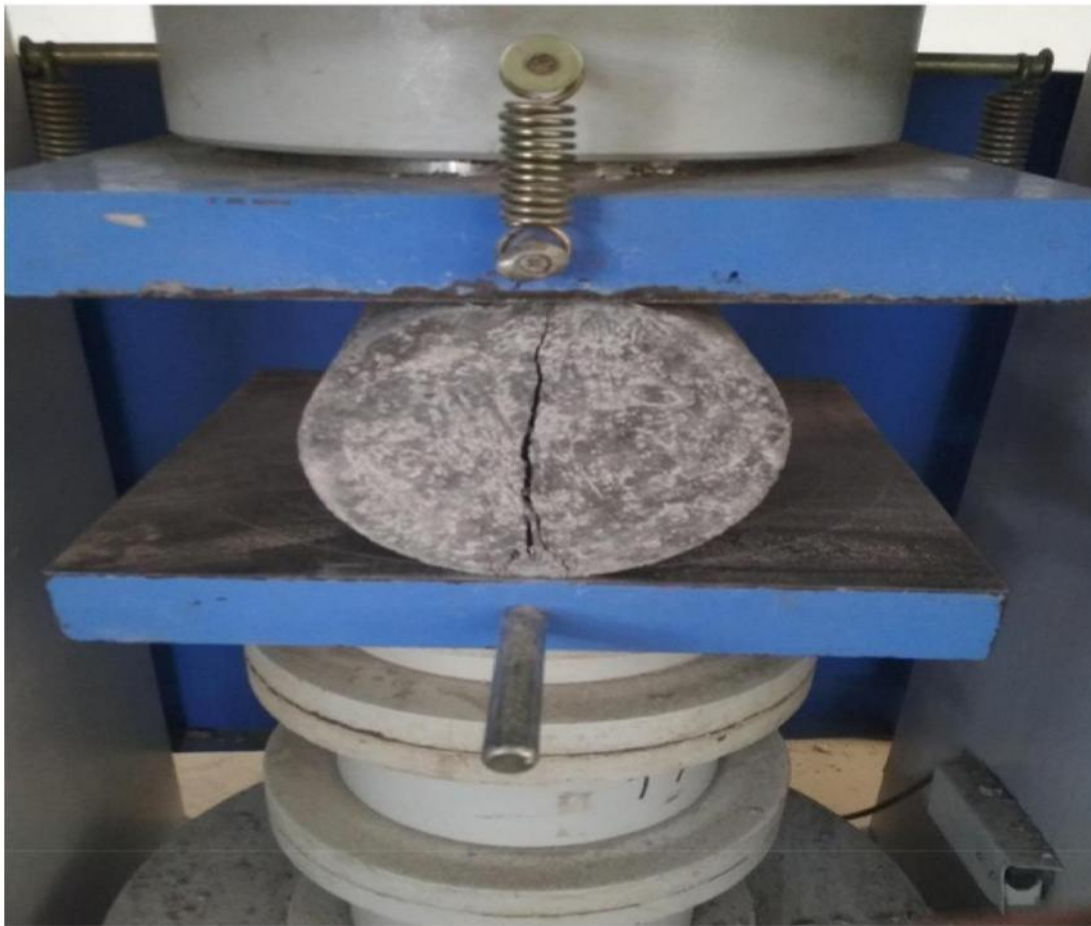
Plate 3.4: Splitting T. strength test of cylinder.
