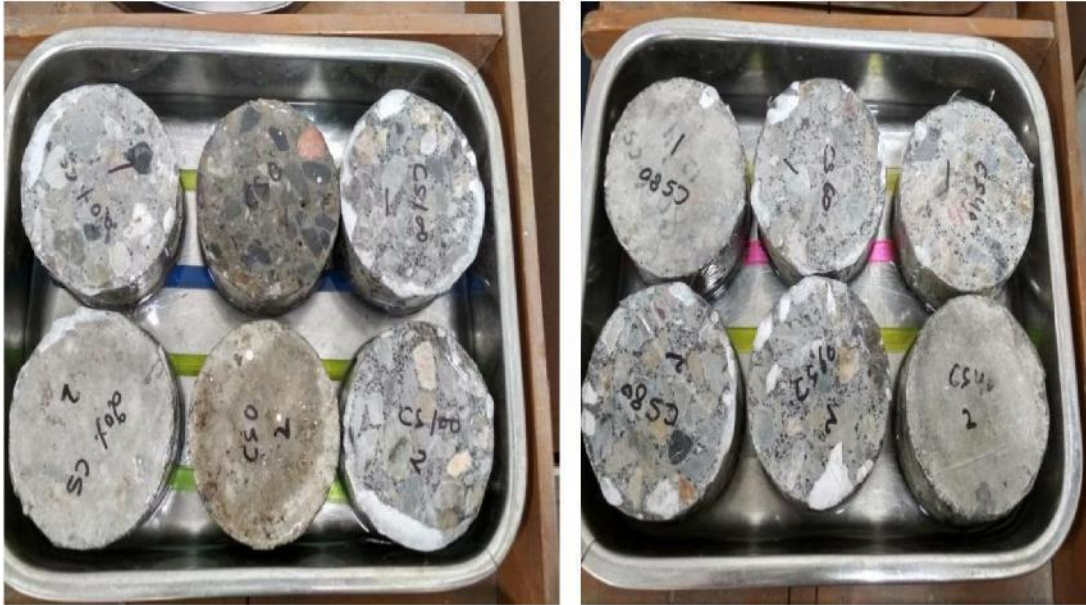
Plate 3.7: Sorptivity test of concrete specimen
