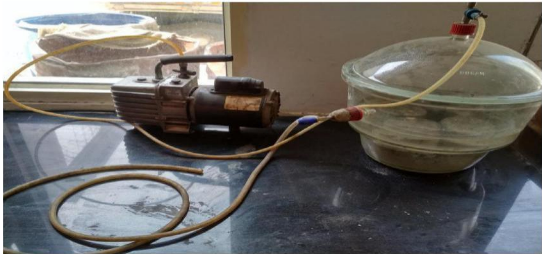
Plate 3.6: concrete specimens placed in desiccator
