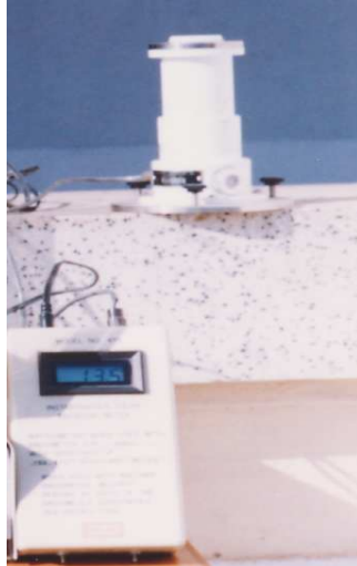
Fig 10. Eppley (model no. 33013) radiometer was used for measuring the UV intensity.
