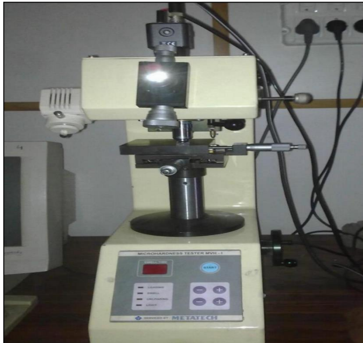
Figure 3.5: Micro hardness testing machine Model: MVH2 (Courtesy: Advance Measurement Lab, Thapar university, Patiala)
