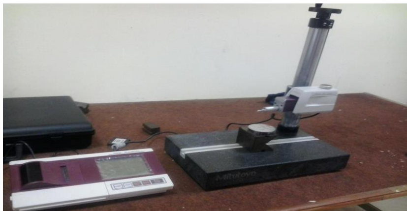
Figure3.6: Surface roughness tester SJ-400 (Courtesy: Metrology lab Thapar university, Patiala)
