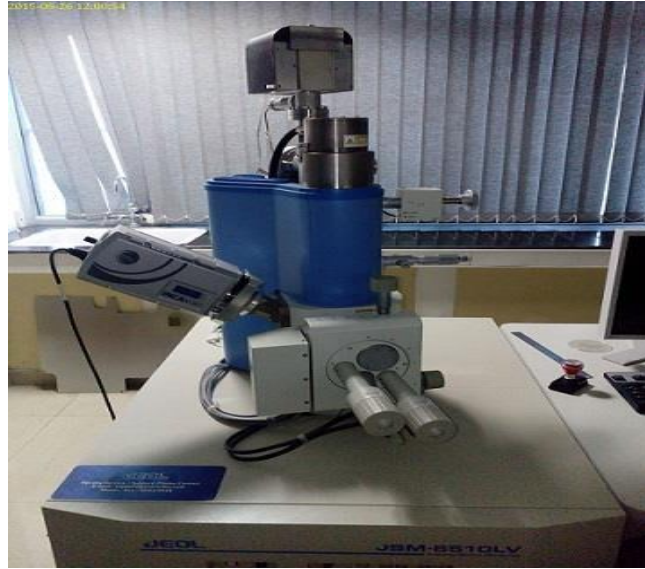
Figure 3.8: Scanning electron microscope (Courtesy: SAI Lab, Thapar University, Patiala)
