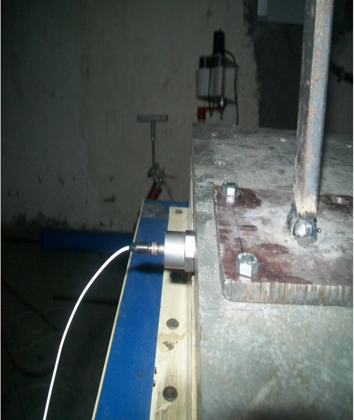
Figure 3.3 Beam mounted on combo base slip table of electro-dynamic shaker
