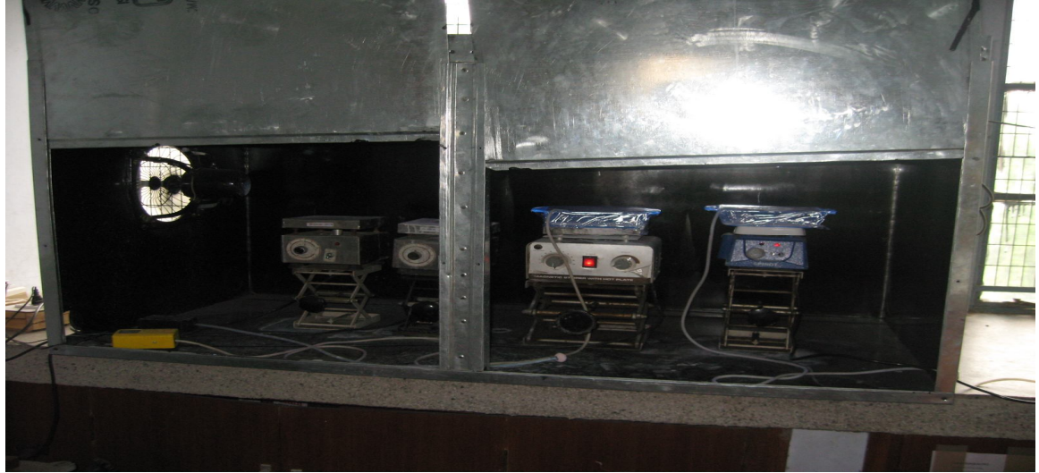
Fig: 4.1.2 Photo reactor at lab level during photo Fenton treatment
