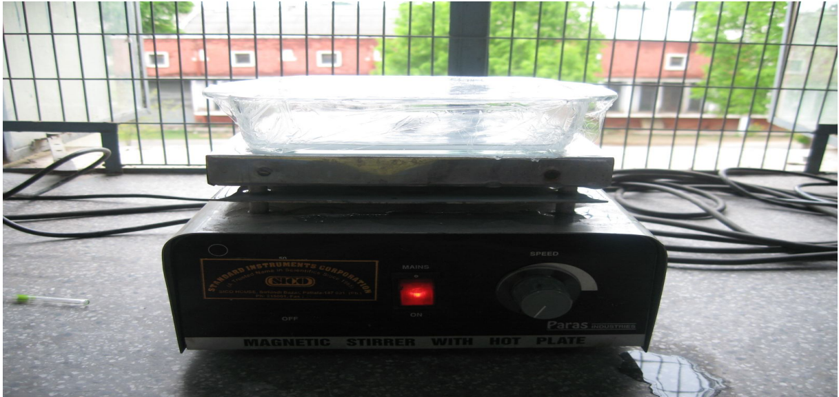
Fig: 4.1.3 Reaction vessel with magnetic stirrer during Fenton treatment.
