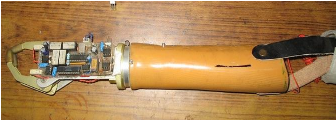
Fig. 1.6 Surface EMG based Myoelectric arm
