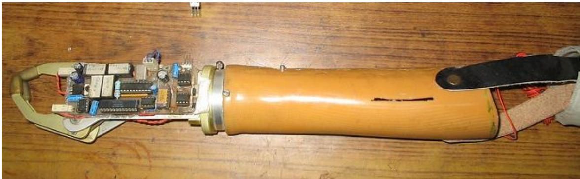
Fig. 6.10 Below-elbow myoelectric arm
