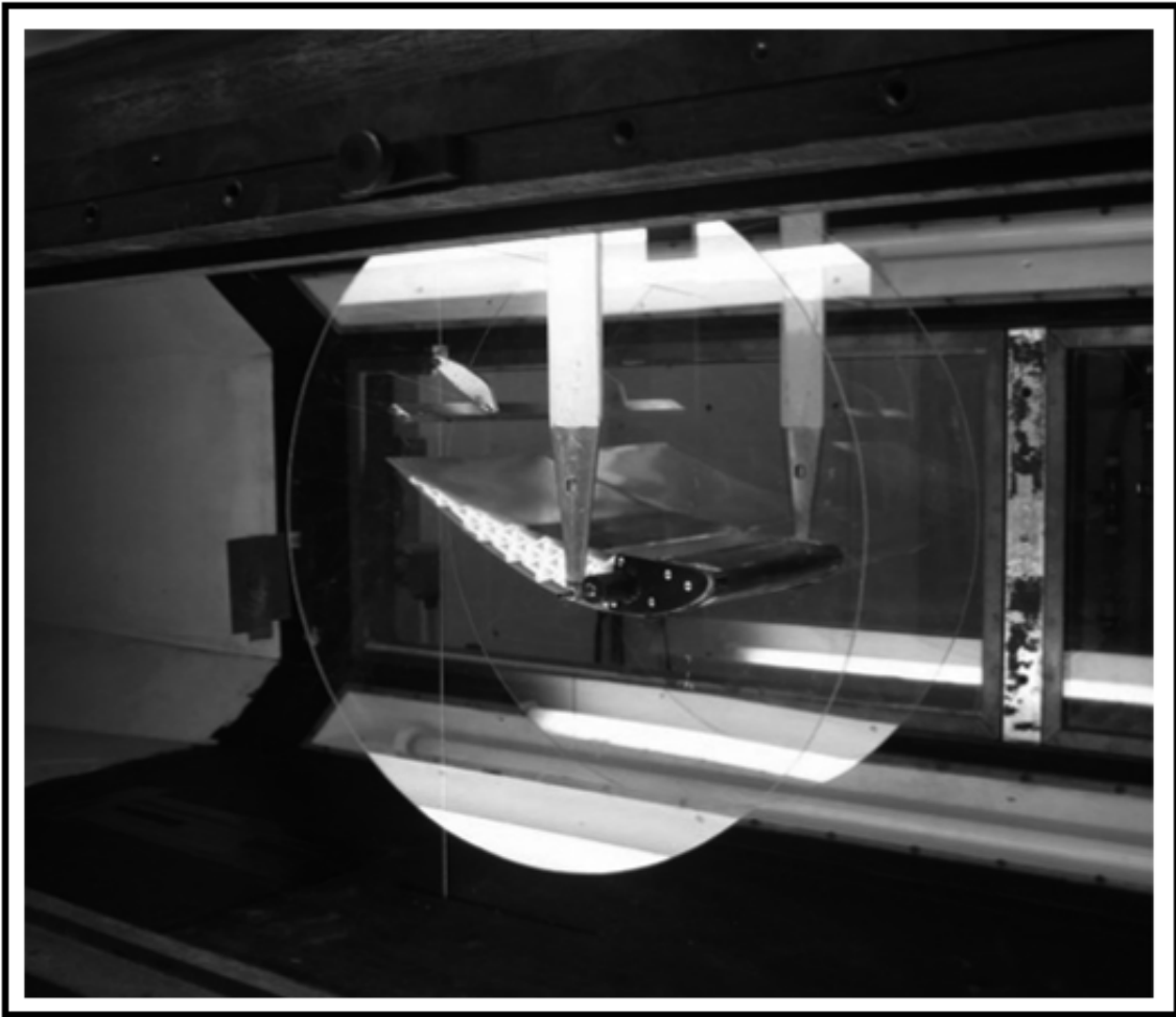
FIGURE 2.18: The proposed prototype of the Wingbox mounted in a low-turbulence wind tunnel [65].
