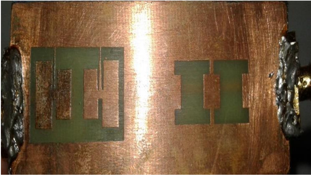
Fig. 5.20 Bottom view of the fabricated Band Pass filter for S-Band applications
