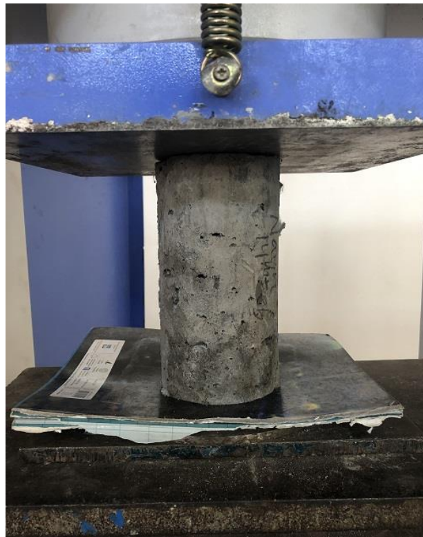
Figure 3.8 Compressive Strength Testing of ECC Trial in Compression Testing Machine
