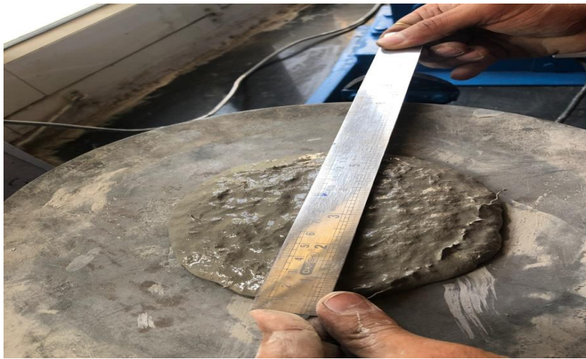
Figure 3.10 Measuring Followability of Fresh ECC
