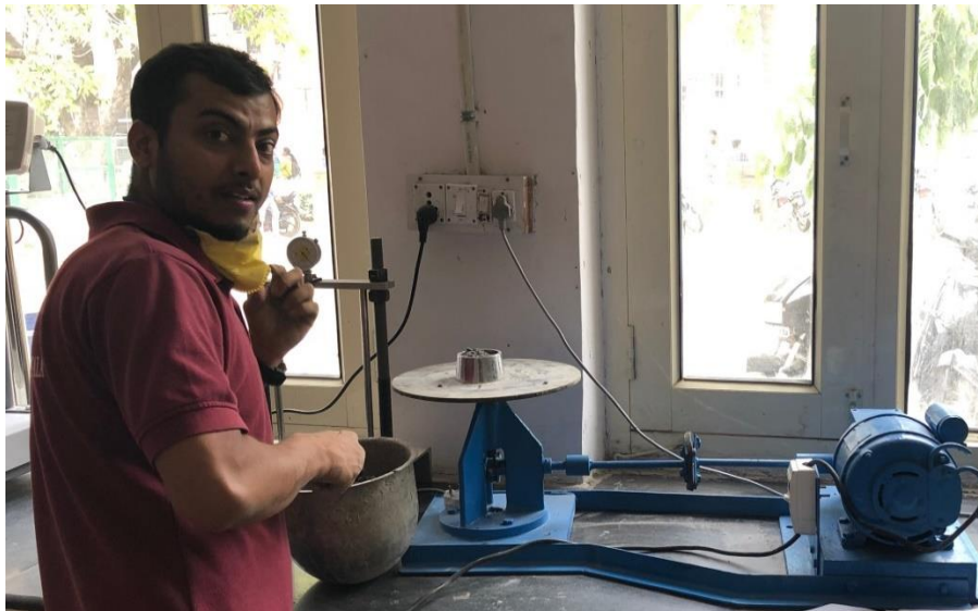
Figure 3.9 Flow Table Apparatus Used in The Study.
