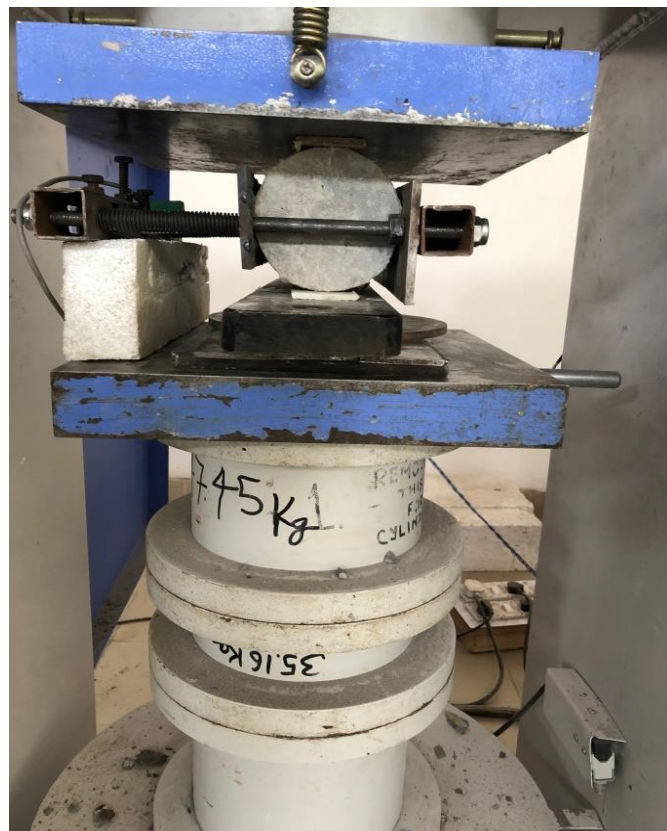
Figure 3.13 Splitting Tensile Strength and Strain Measuring in CTM
