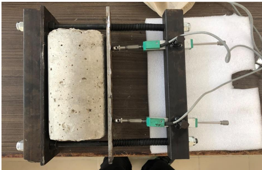
Figure 3.11 Split Tensile Strain Measuring System
