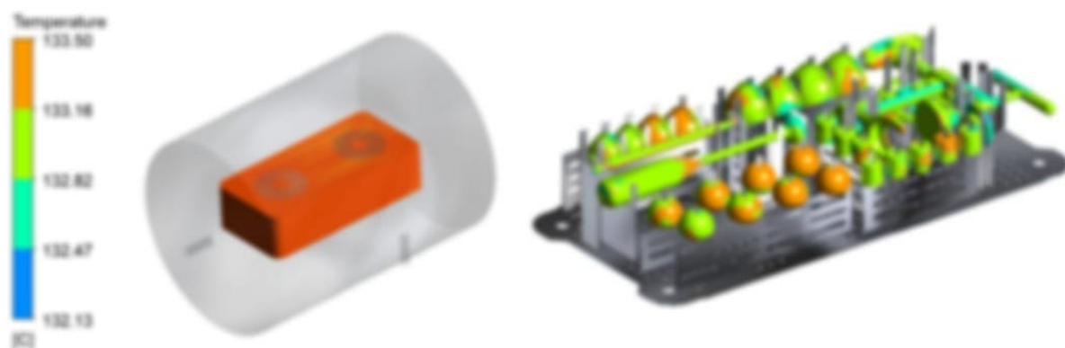
Figure 5-7 Temperature Distribution of the Surgical Instruments after 240 seconds
