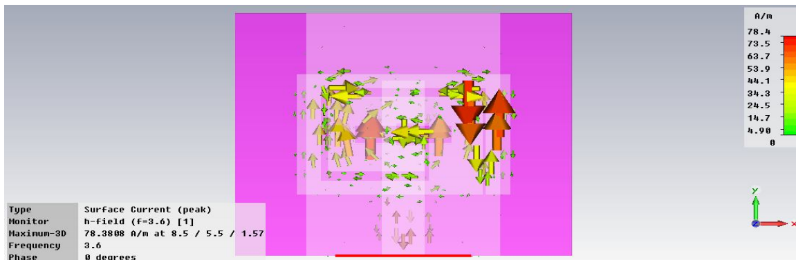
Figure 4.6: Surface current of the antenna at 3.6 GHz.
