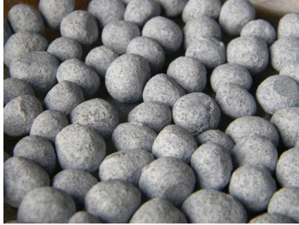
Figure 3.4: TiO 2 coated cement beads used for the degradation studies
