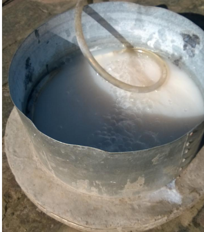
Figure 4.44: Pilot-scale slurry batch reactor
