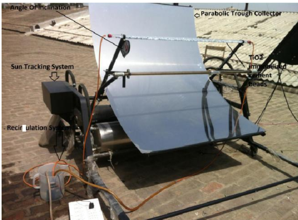
Figure 3.7: (a) Schematic diagram of parabolic trough collector (b) Actual site photograph of Parabolic Trough collector.
