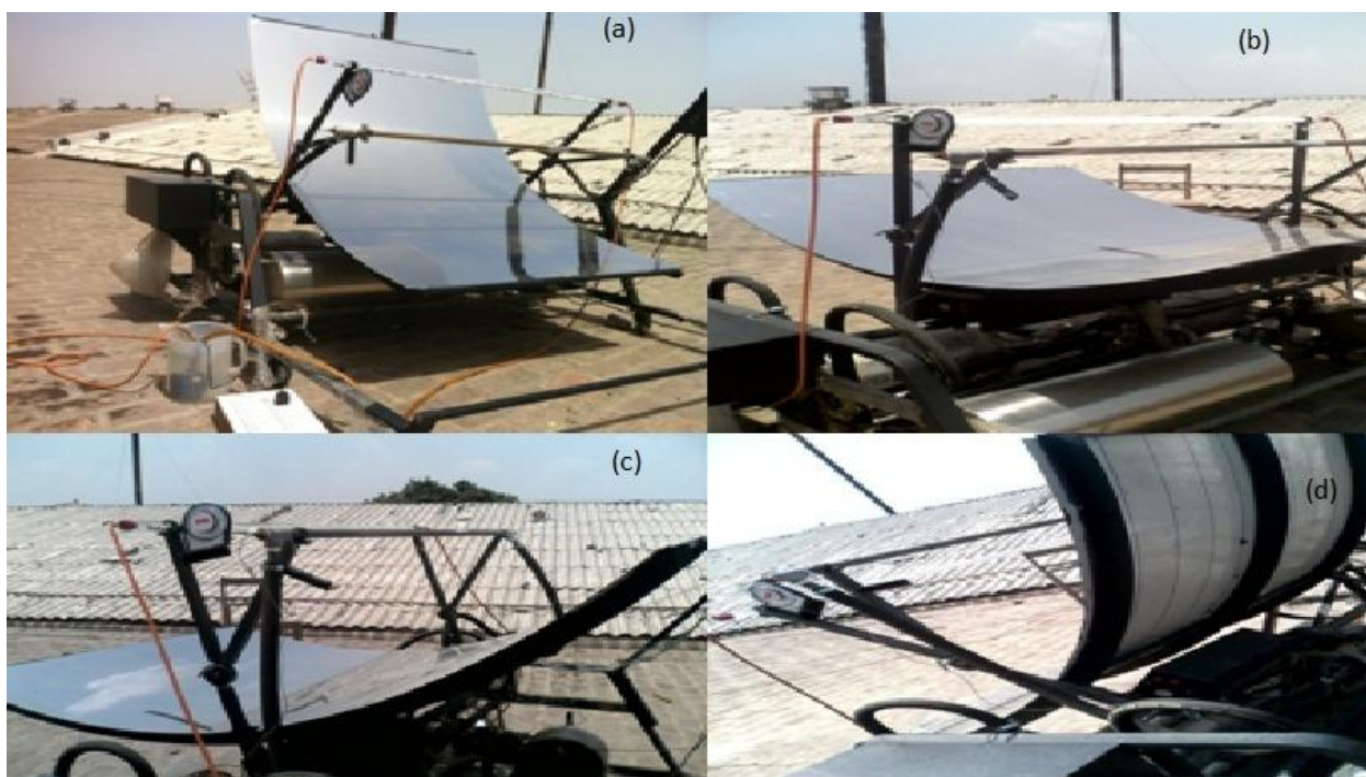
Figure 4.48: Representation of Solar Parabolic Collector at the angle of inclination of (a) -40^\circ (b) 0^\circ (c) 20^\circ (d) 40^\circ respectively.
