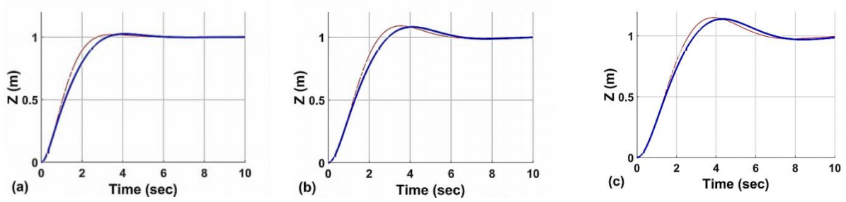
Figure 5.29: Response of z position for pendulum mass ( m ) in kg = a) 0.1; b) 0.8; c) 1.5 (solid line: robust LQR based ANFIS controller and dashed line: LQR controller)
