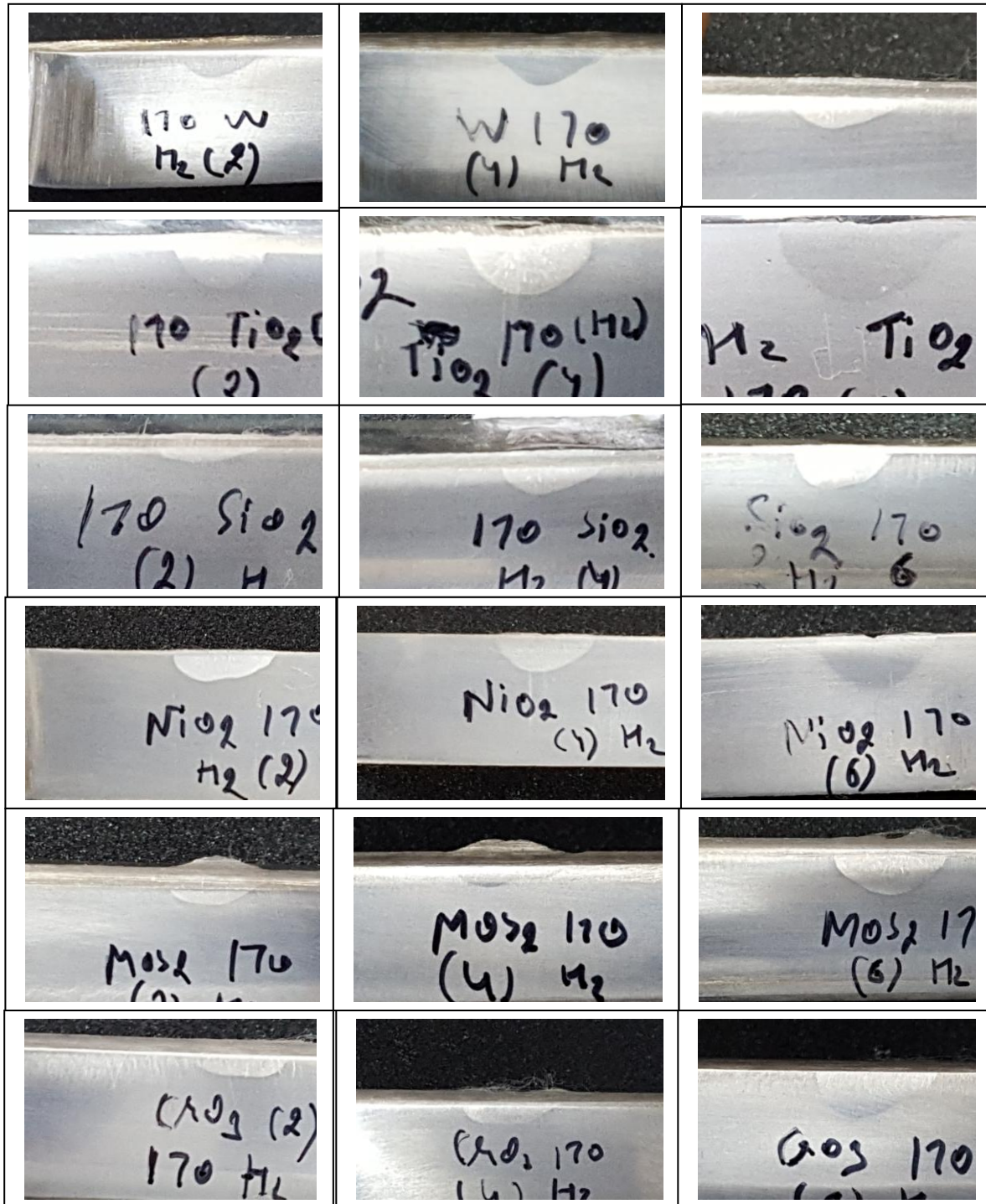
Figure 4.9: weld bead appearance for TIG and ATIG welding
