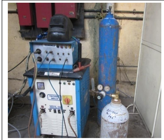
Figure 3.2: welding setup for TIG
