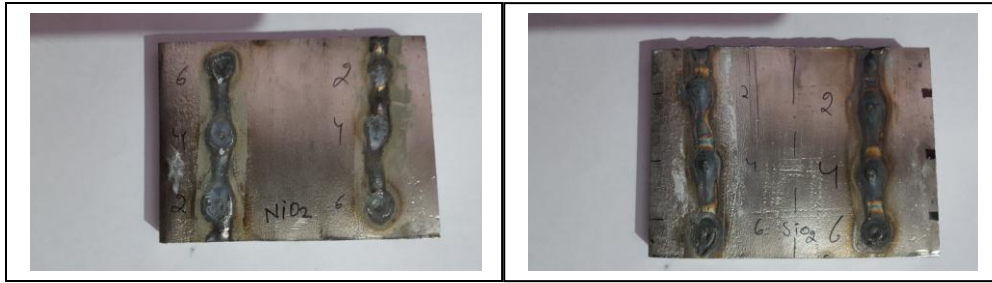
Figure 3.4: Welding bead appearance on surface of work pieces using flux and without flux for 2 sec, 4 sec and 6 sec (at current- 190 A).
