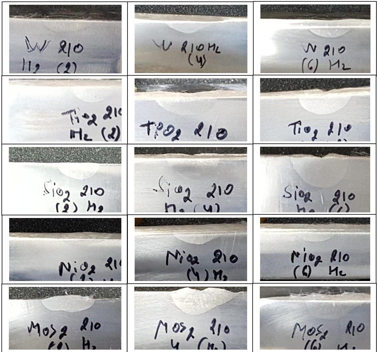
Figure 4.13 Bead appearances for TIG and ATIG welding at 210 A current.
