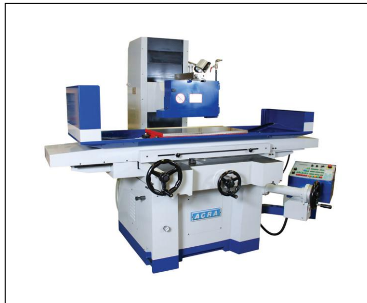
Figure 3.5: Surface grinder ( www.ronmack.com.au )
