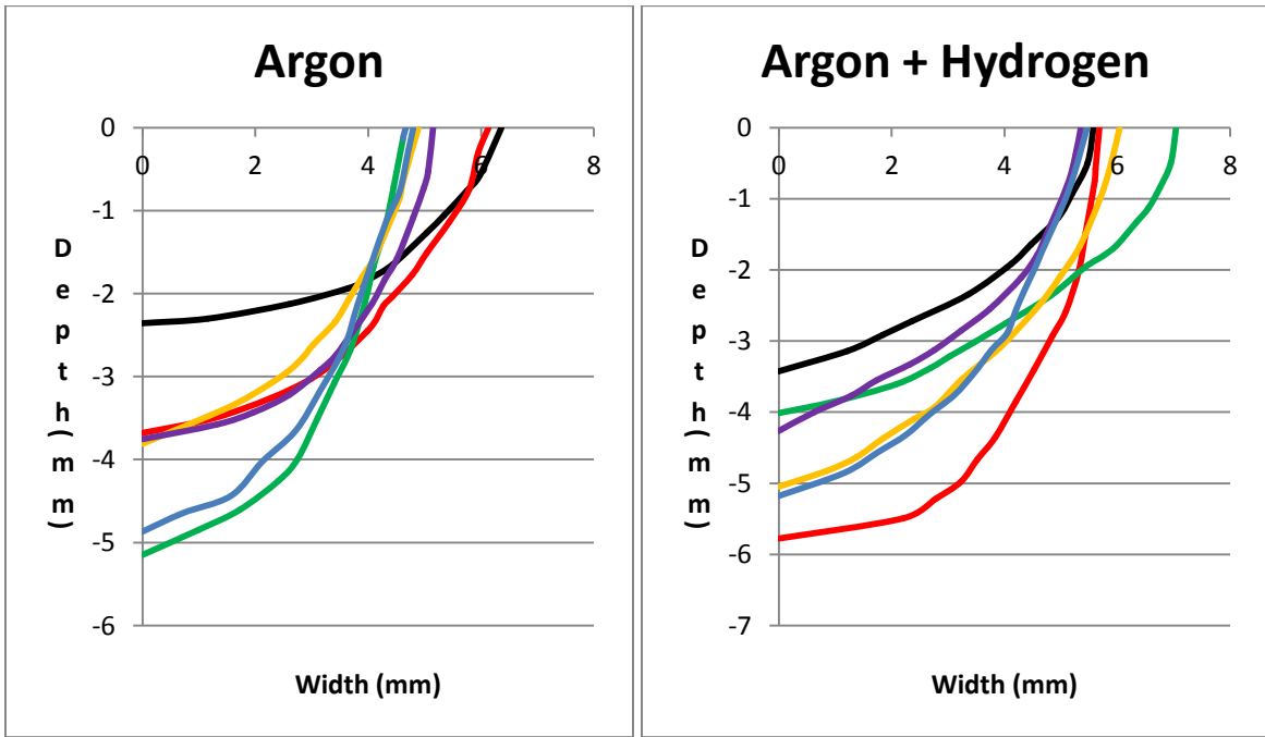
Figure 4.22: Comparison between both types of shielding gas for 6 sec and current- 210 A (Black- without flux, Blue- TiO 2 , Red- SiO 2 , Green- NiO 2 , Orange- MoS 2 , Purple- CrO 3 )
