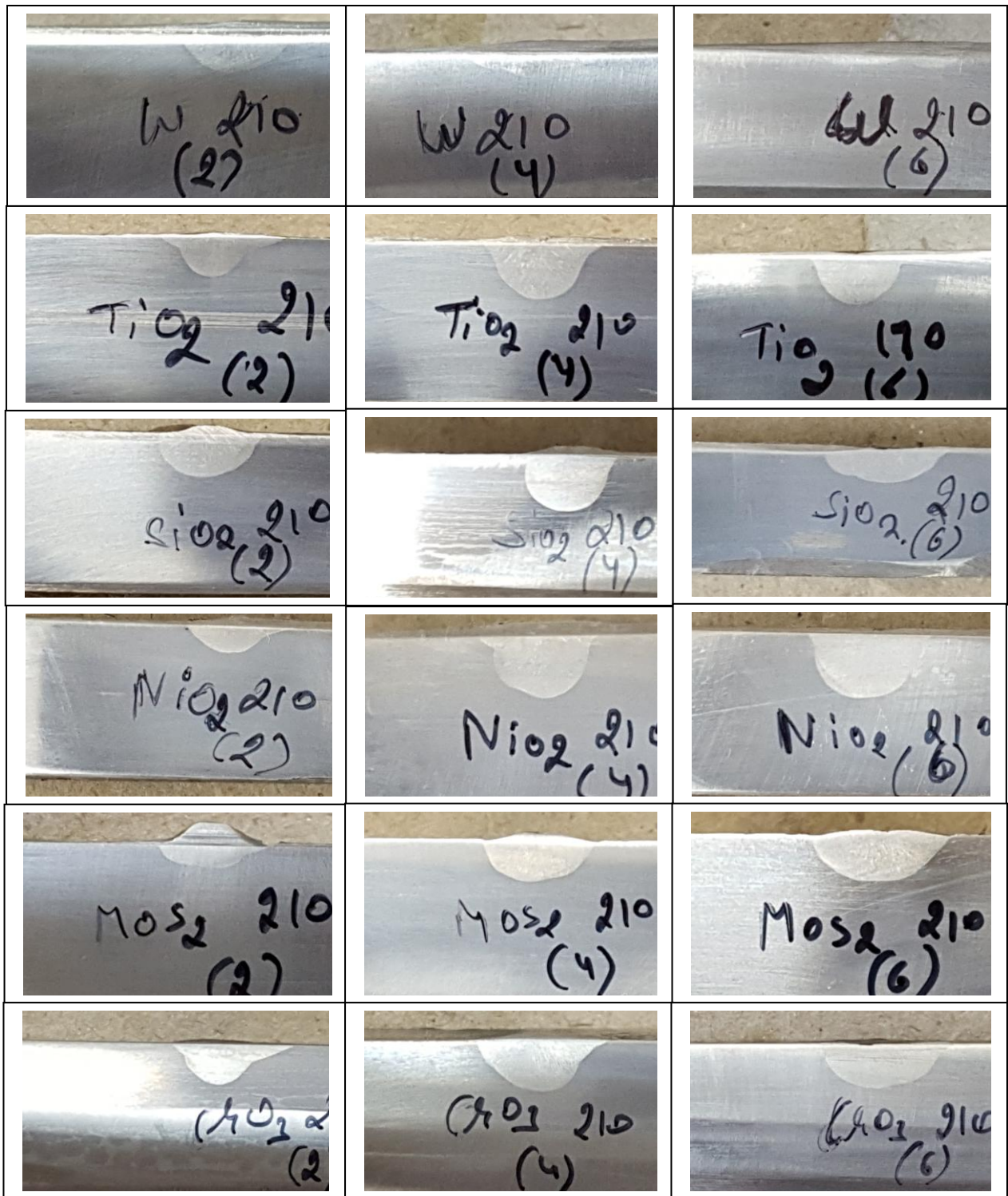
Figure 4.7: Bead appearance for TIG and ATIG welding samples for 2 sec, 4 sec and 6 sec at current- 210 A
