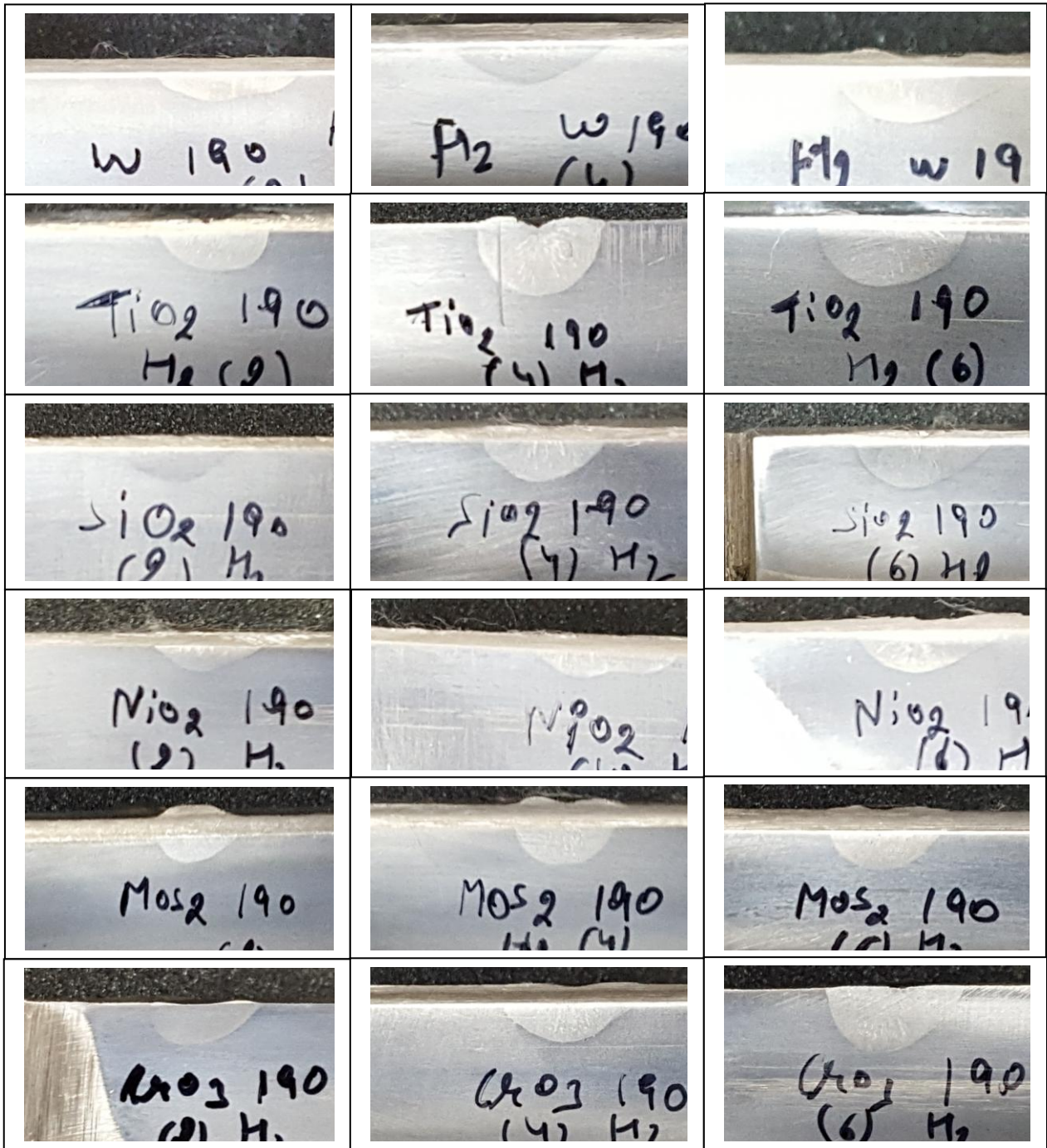
Figure 4.11: Bead appearance of TIG and ATIG welding at 190 A of current
