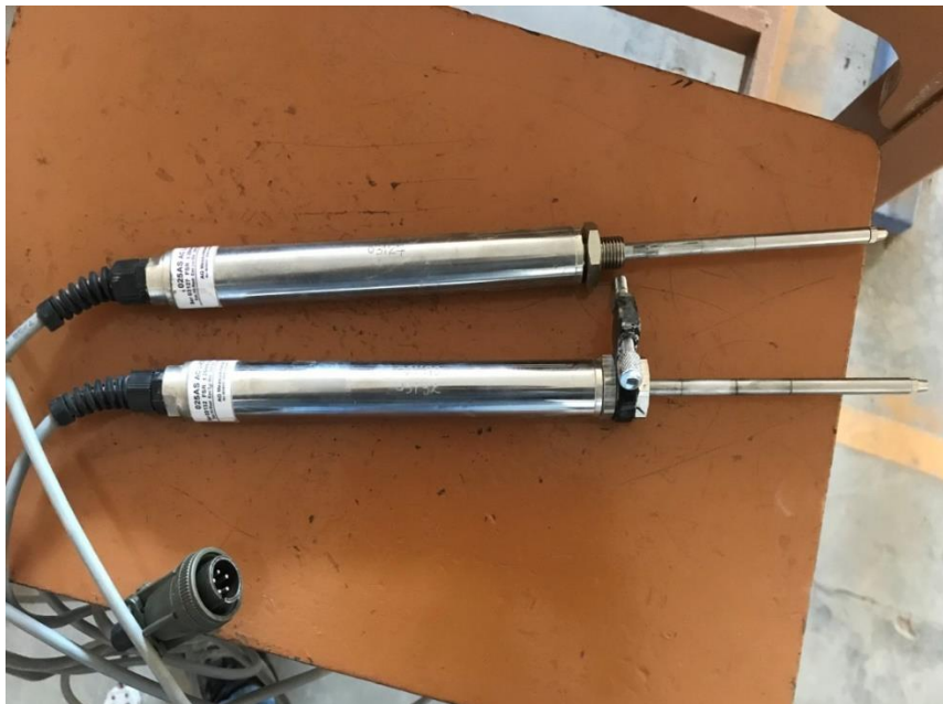
Figure 3.6: AG Measurematics Alternating Current LVDT.
