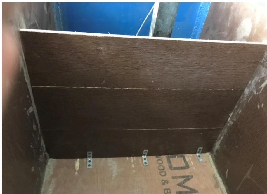
Figure 3.5: 12 mm thick 3 panelled reduced friction wall.
