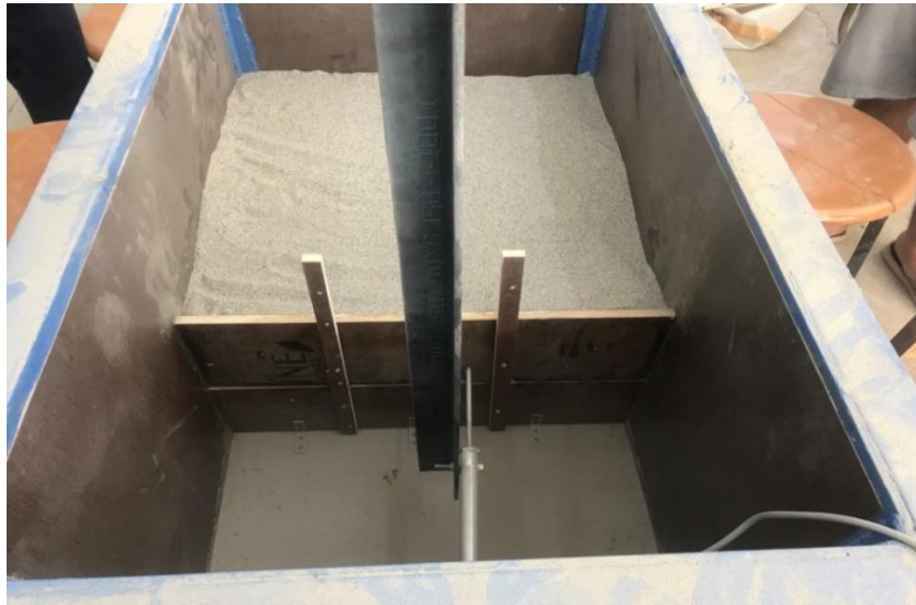
Figure 3.4: 12 mm thick 3 panelled staged wall.
