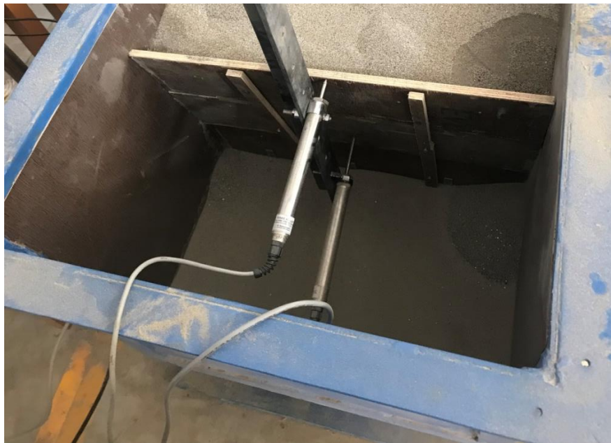
Figure 3.15: Attached LVDT's to the metal frame.
