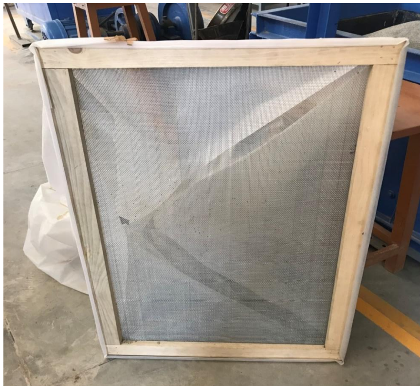
Figure 3.10: Custom made sieve of size 1.75 mm.
