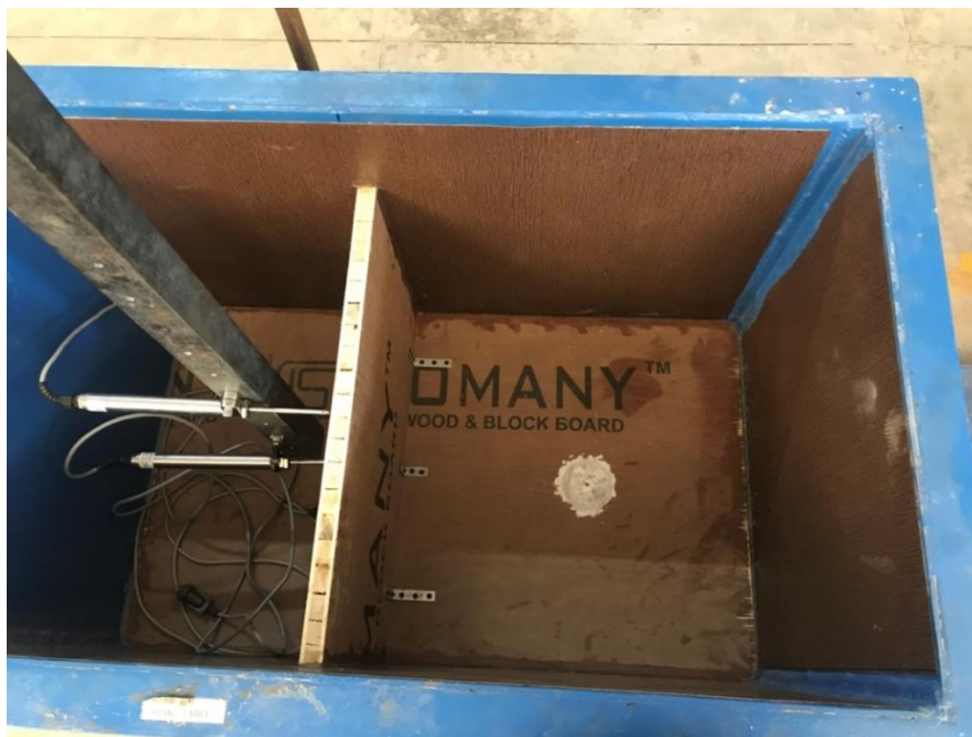
Figure 3.14: Plywood Base of the Shaking Table.
