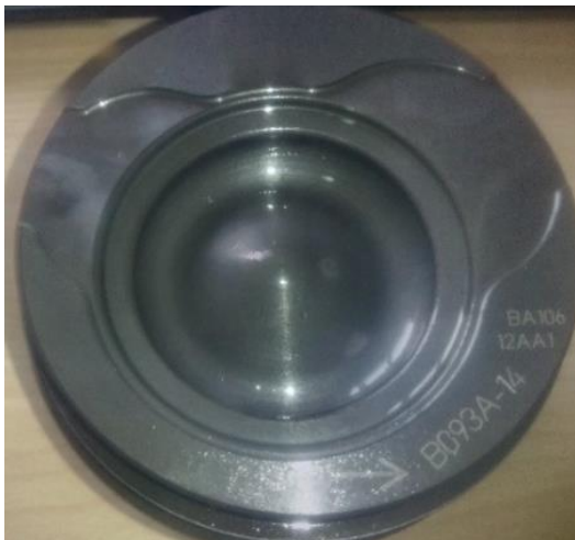
Fig. 28 Manufactured modified piston CR 17.11:1
