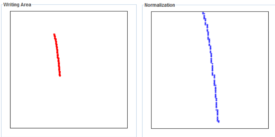
Figure 3.19: Slanted line (negative slope) problem corrected
