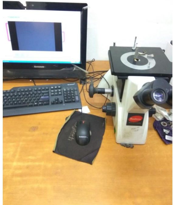
Fig 5.2: Digital Microscope used for metallurgical examination (23)
