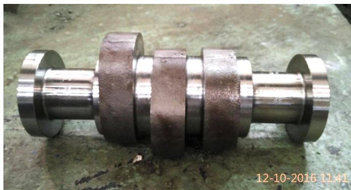
Fig 5.9: A proof machined forging adopted for manufacturing of Stiffer Unit Camshafts
