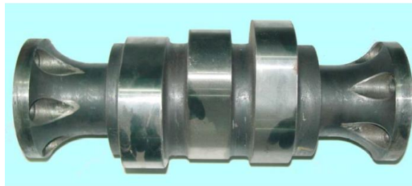
Fig: 1.6 New Design Stiffer Unit Camshaft with Base Circle Dia of 160 mm (11)
