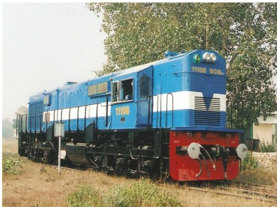
2600 HP WDM 2 ALCO Locomotives (16 Cylinder V Engines)
