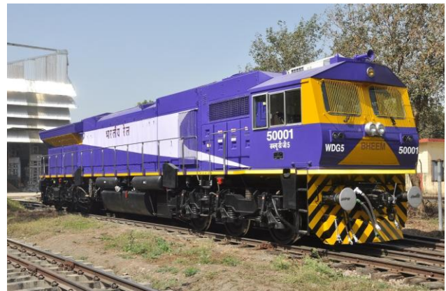
4500-5500 HP WDG 4/5 EMD Locomotives (20/24 Cylinder V- Engines)
