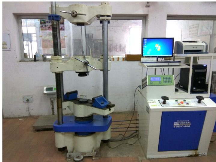
Fig 5.7 : Computerised Universal Testing Machine, Model TUE-C-400 available in the DMW Laboratory used for testing of Mechanical Properties of the samples (23)
