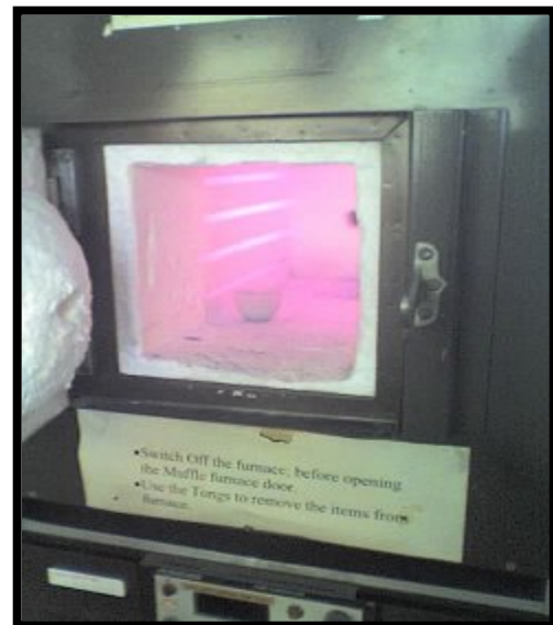
Figure 4.2 Figure showing fuel sample being placed in muffle furnace
