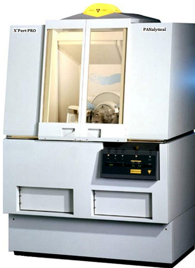
Figure 2.6 Photograph of x-ray diffractometer by PANalytical X'Pert PRO MPD
