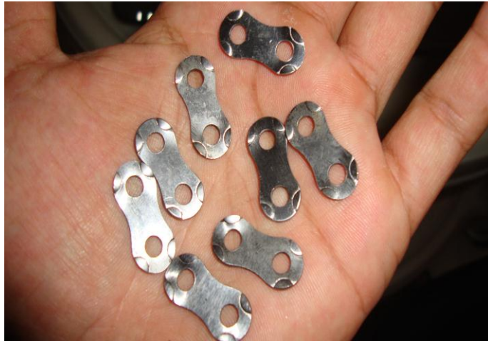
Figure 3. 16 :- Embossed outer link plates of chain after the embosing tool try-out at Central Tool Room, Ludhiana
