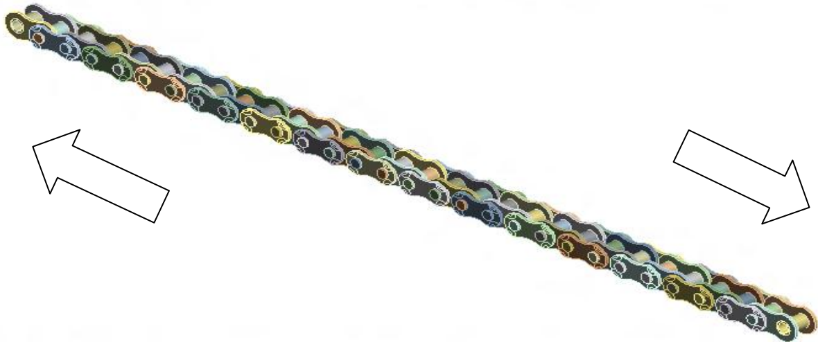
Figure 3. 9: 15 Links chain used for Tensile Testing.
