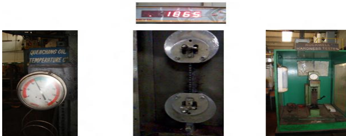
Figure 3. 19 Quenching oil temperature 50-80° C, UTM Tester and Rockwell hardness tester respectively used in rock man industries
