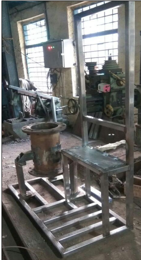
Figure 15 Tack welded skid
