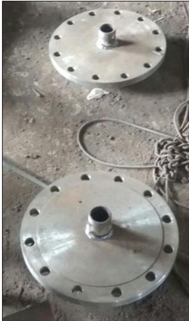
Figure 16 Flanges for reactor base and top
