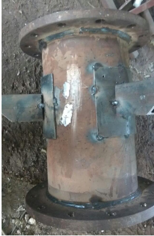
Figure 13 Fabricated reactor anoxic Part
