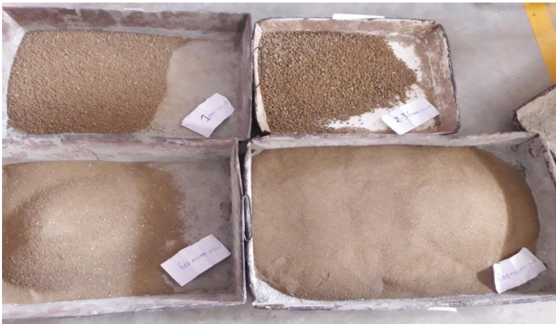
Figure 4: Different grain sizes of soil particles
