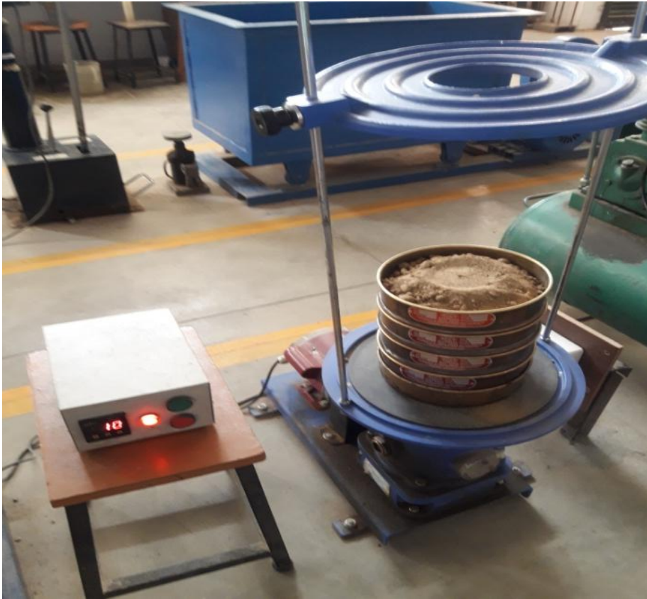
Figure 3: Mechanical shaker used for sieve analysis
