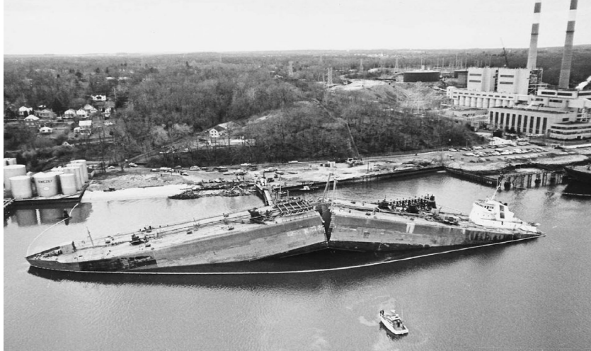
Fig 2.5 Fracture of ship due to ductile to brittle transition
