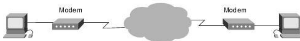
Figure 1.10A Modem Connection through a WAN Handles Analog and Digital Signal [17]
