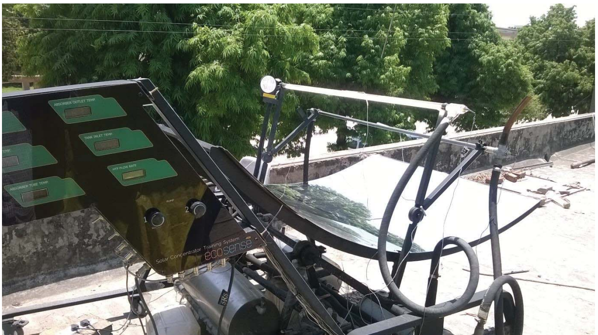
Figure 3.1 Parabolic trough collector
