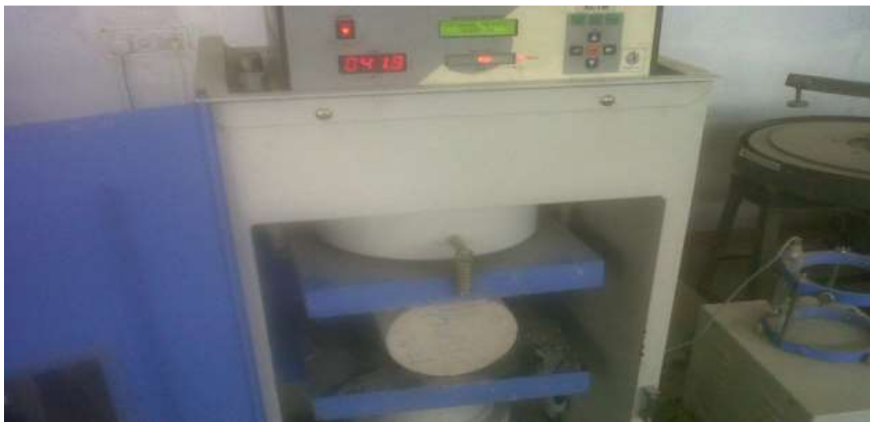
Figure 4.3 Split tensile test in laboratory
