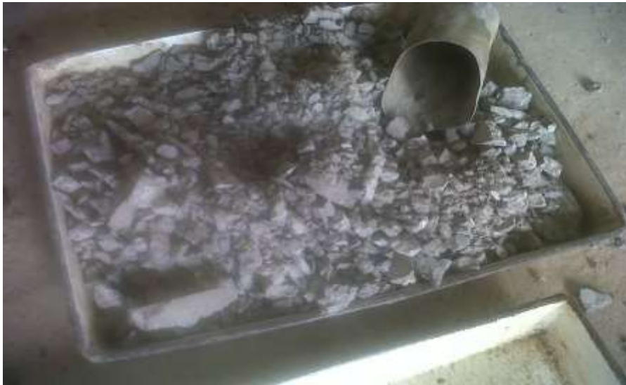
Figure 1.1 Recycled concrete aggregate size 10-30mm
