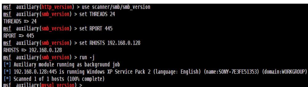
Fig.39: Services running on ports and OS running on host.
